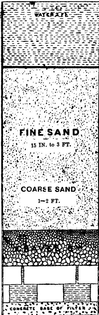
FIG. 8-i. SECTION of a SAND FILTER (After Knight's Diagrammettes).
