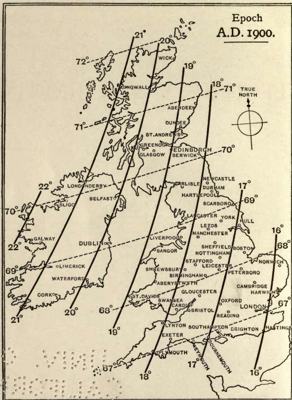
MAGNETIC CHART OF THE BRITISH ISLANDS, SHOWING THE LINES OF EQUAL MAGNETIC DECLINATION AND THOSE OF EQUAL MAGNETIC DIP.
