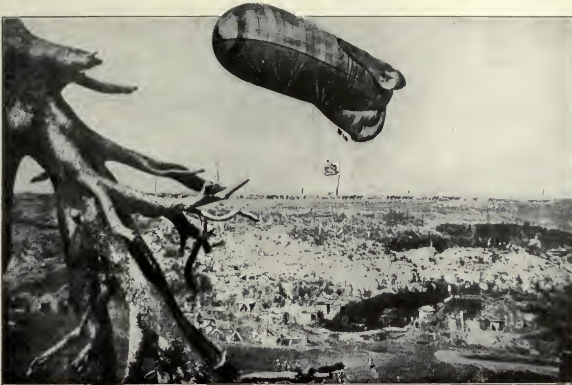
A French captive balloon of the Caquot type just behind the firing lines.
