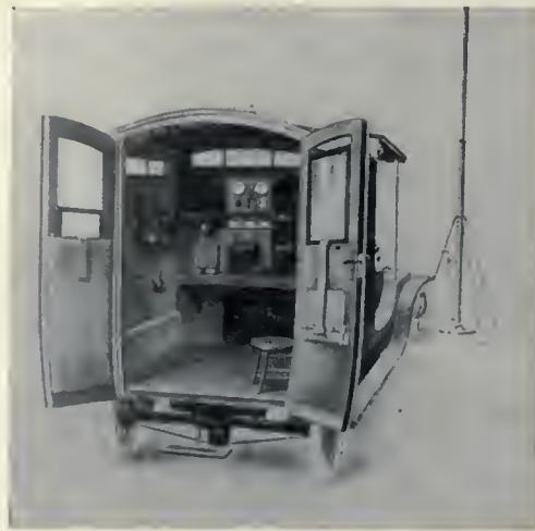
Fig. 12. A motor car wireless station.
