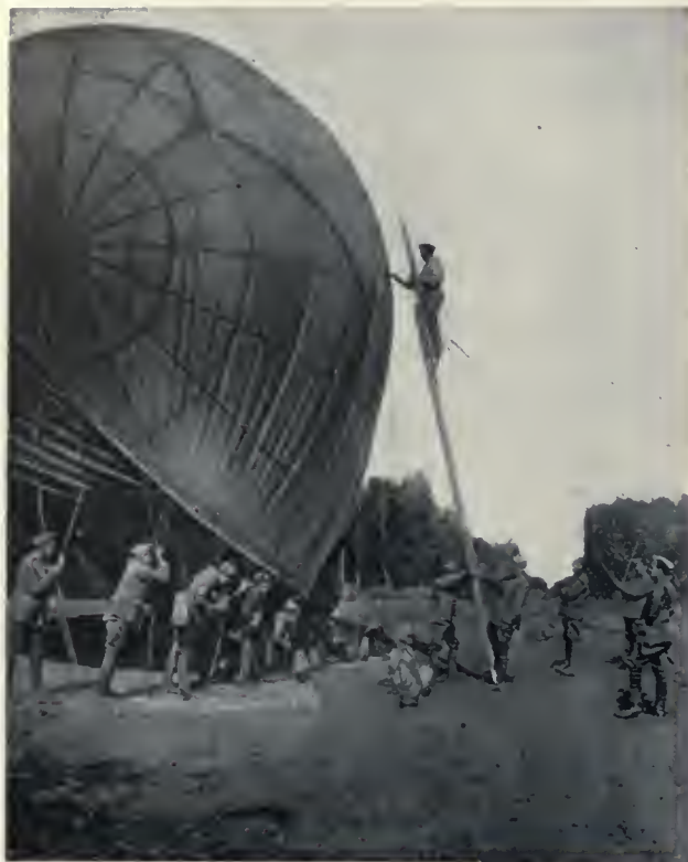
Members of the Canadian Kite Balloon Section patching up a kite balloon on the Somme front.
