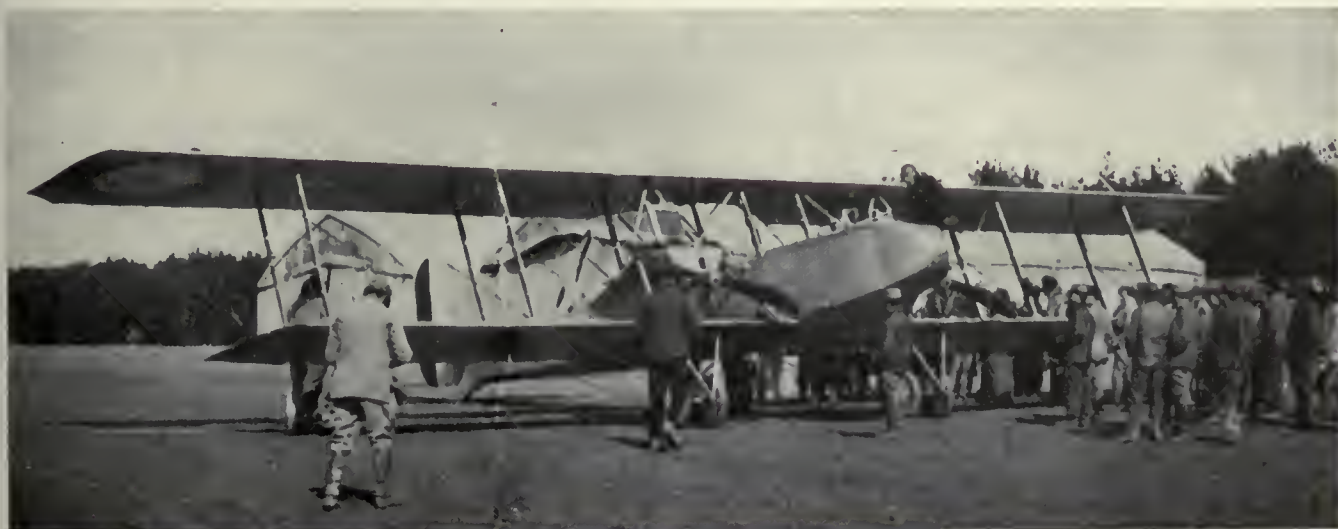
The French "Corps d'Armée" type, "Letort" battleplane equipped with two 150 h.p. Hispano-Suiza motors and mounting two Lewis and two Vickers guns.
