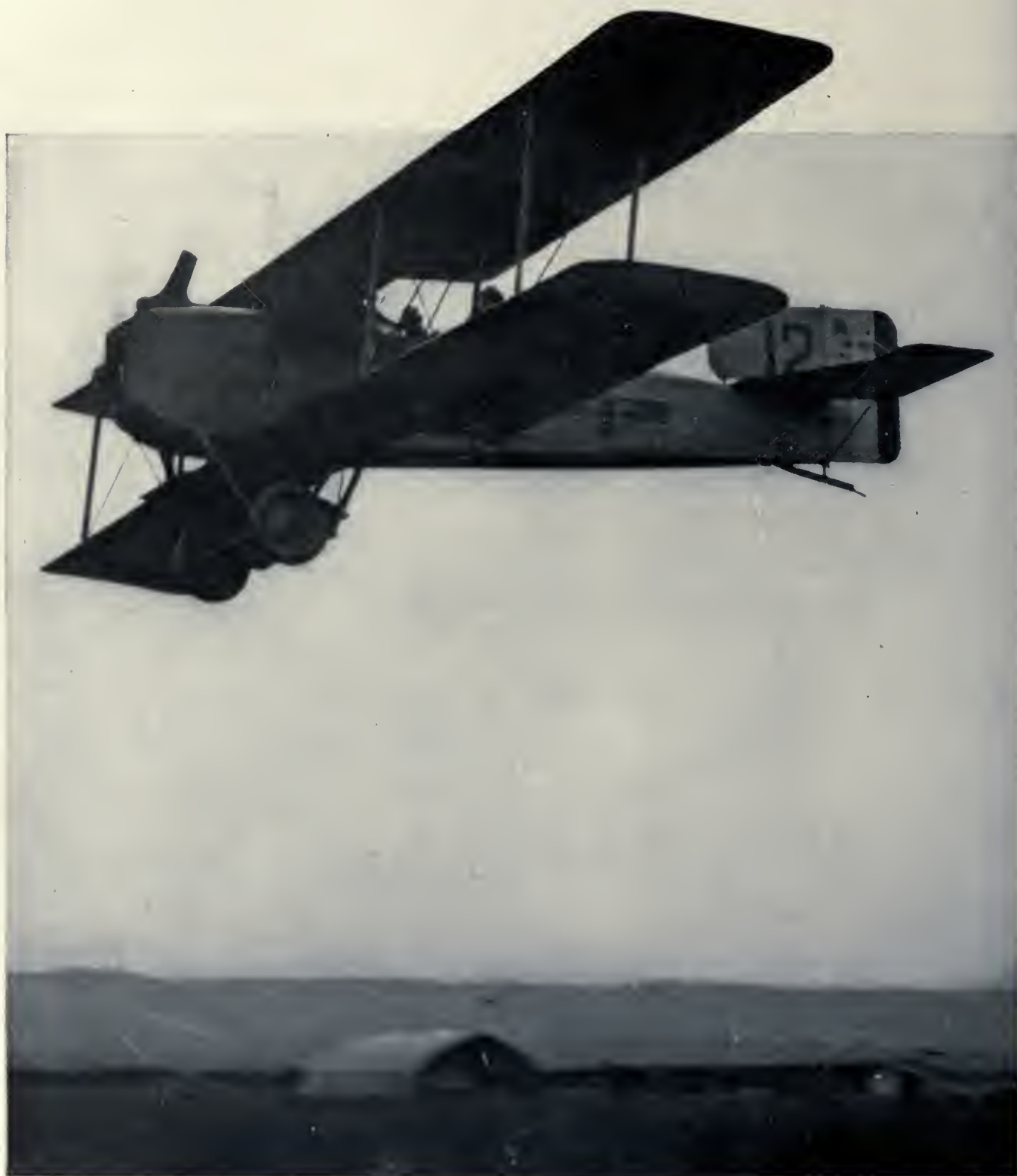
One of the Breguet bombing type biplanes used by the French, which are most remarkable climbers, though they are limited in the load they can carry. Unfortunately the Germans have brought down several of this type and will be able to copy it. (French Official Photo.)
