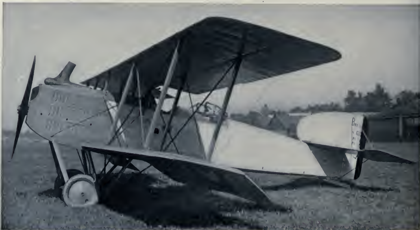
A French Breguet tractor biplane used for bombing, photographing and artillery spotting.
