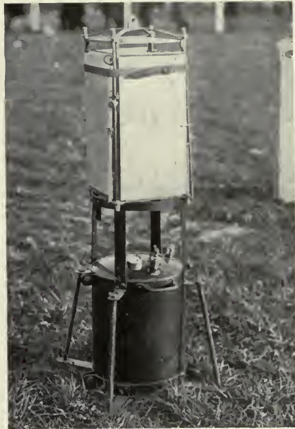
Portable aerial beacon of 2400 decimal C.P.
