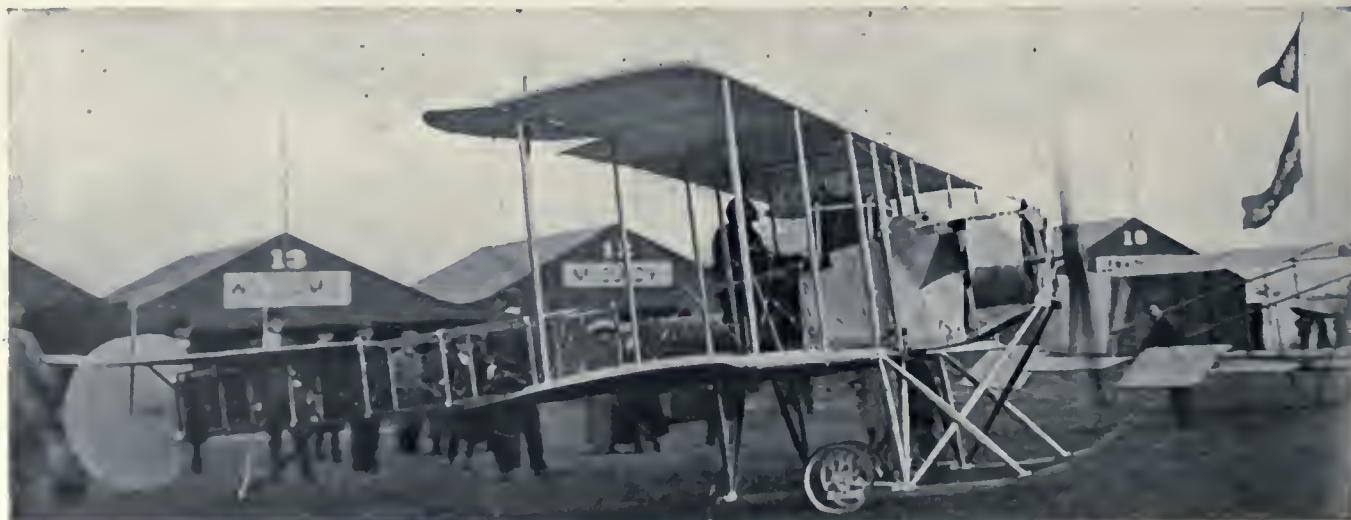
The first tractor biplane in America. Constructed by Captain James V. Martin in August, 1911. The first flight took place in November, 1911, at Nassau Boulevard, L. I. It was equipped with a 100 h.p. Gnome motor.
