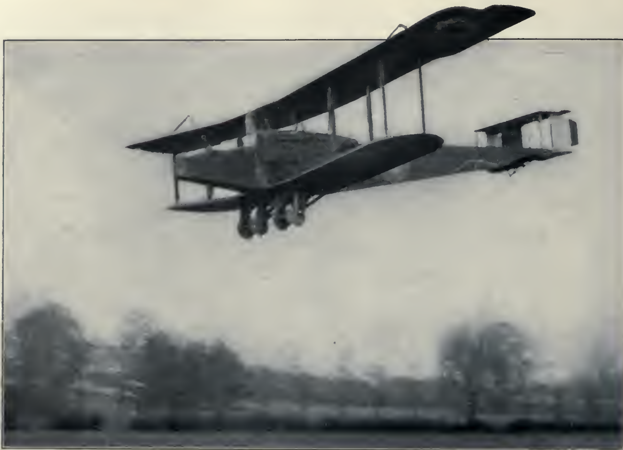
The Twin-Motored Handley Page Bombing Biplane. A Handley Page has flown from London to Asia Minor, with stops, and dropped bombs on Constantinople. It carried seven men, spare motors and supplies. Larger Handley Pages can fly across the Atlantic and bomb the German bases and munition plants.
