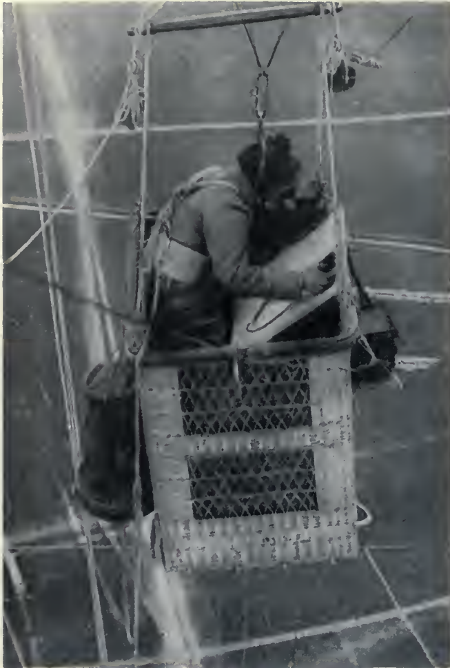
The observer in a captive balloon directing artillery fire. His equipment includes a chart of the sector, divided in squares, which enables him to quickly estimate the accuracy of the firing. He transmits the information to the battery commander who, in turn, orders the gunners to fire according to the information received from the observer.
