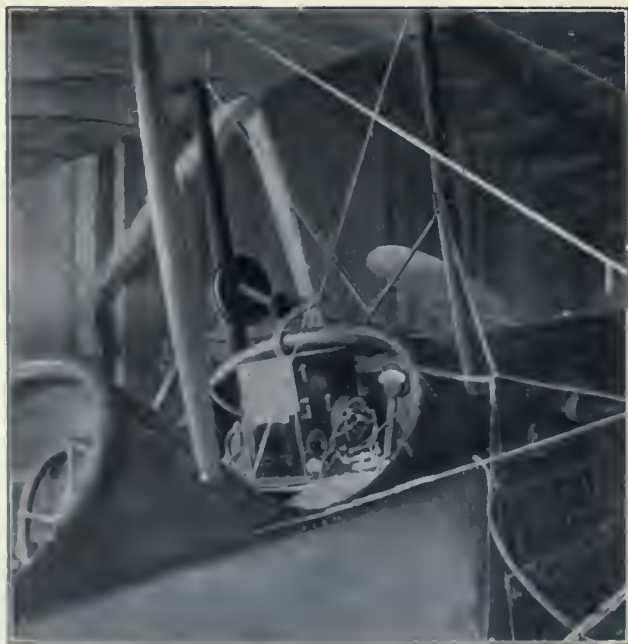
View of the cock-pit, showing arrangement of the Culver set which transmitted 119 miles.
