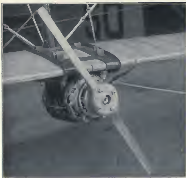
The fan-driven generator, for the Culver set, which furnished power to send messages over a distance of 140 miles.
