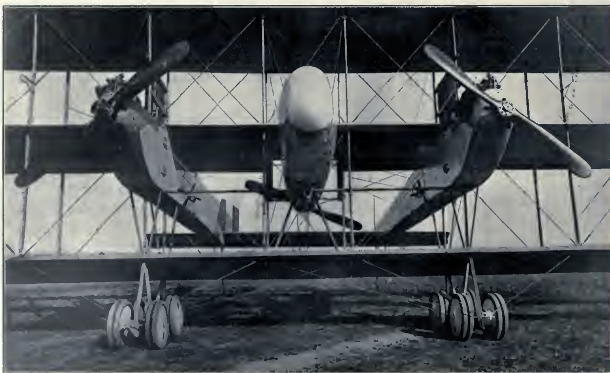
Partial view of the Caproni Triplane equipped with three motors of 200 h.p. This machine has a wing spread of 101 feet.
