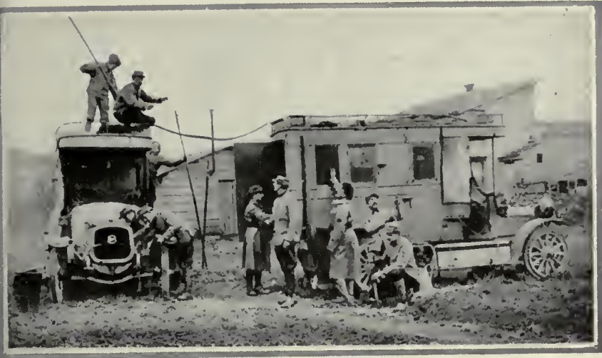
Rigging up the wireless receiving post between two wireless motor trucks "somewhere in France."
