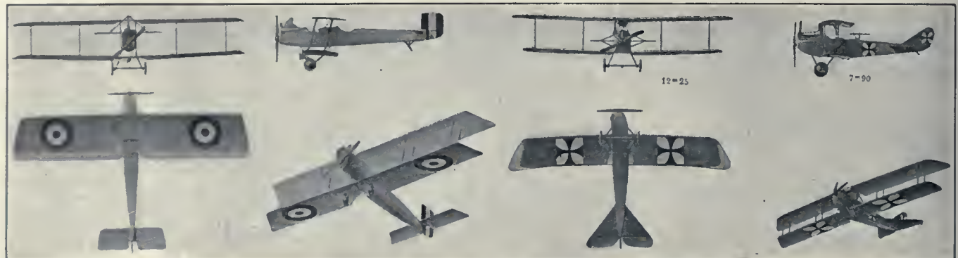
A.R. or A.L.D. French machine for all uses. Planes are invertly staggered and the fuselage is set above the lower plane.
