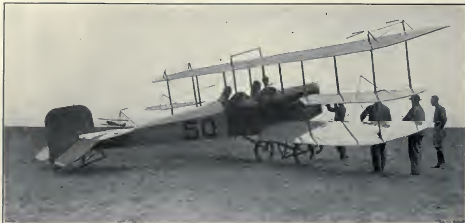
U. S. Army biplane used in Capt. Culver's experiments, showing radio apparatus and aerials.
