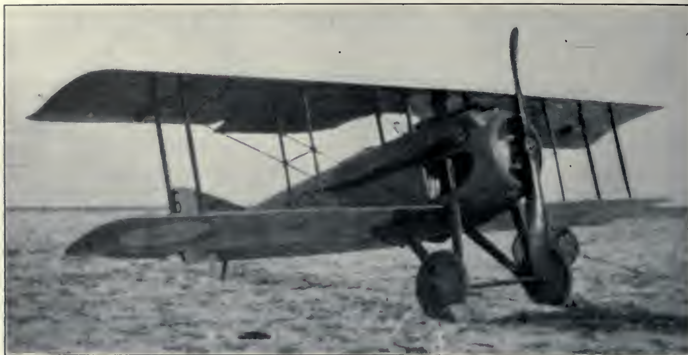
A view of the French "Spad" equipped with the Hispano-Suiza 160 h.p. motor and Vickers gun in front and Lewis in the rear.
