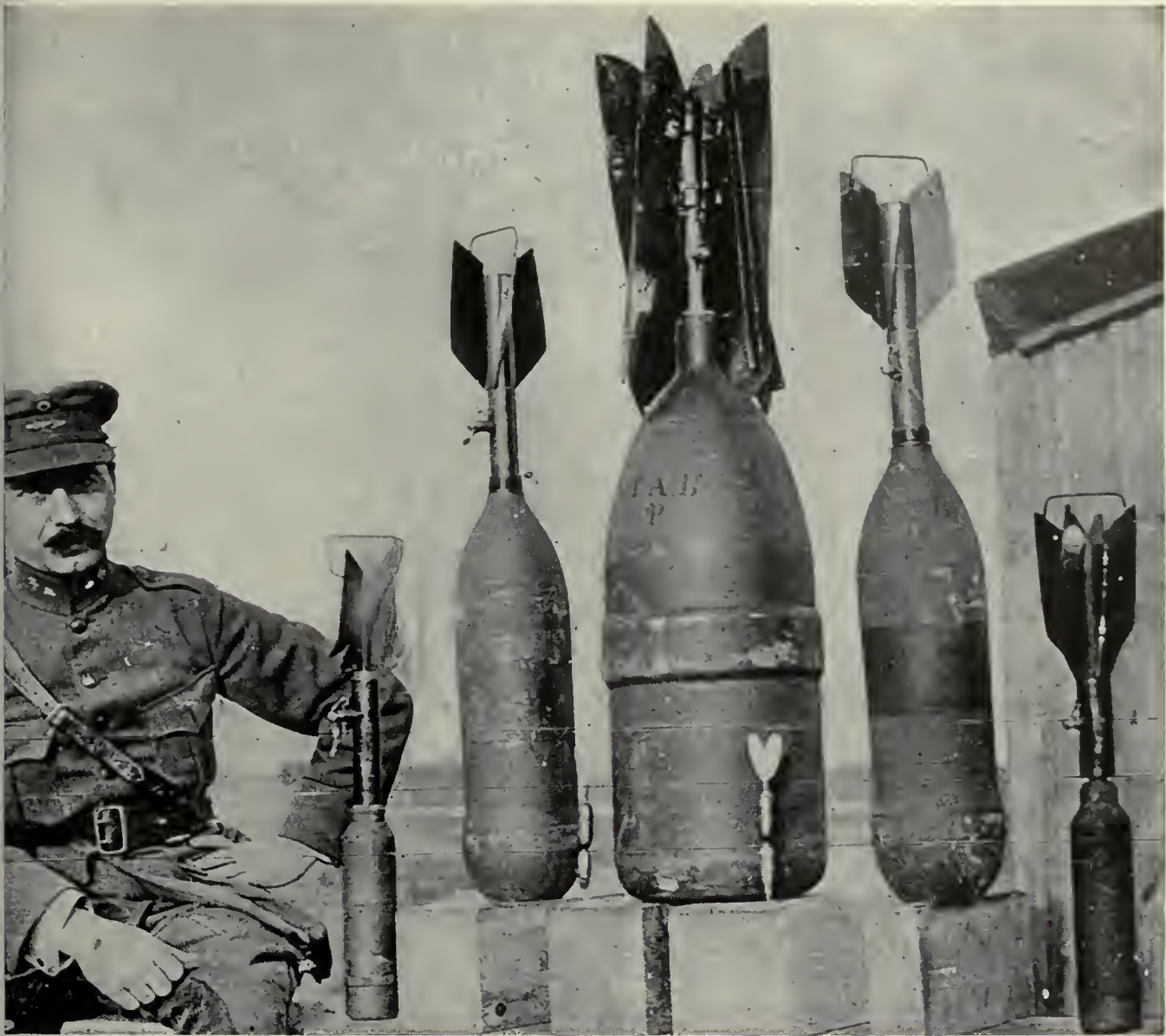
Five different sizes of bombs dropped from aeroplanes. The weight of aeroplane bombs to-day varies from 16 to 500 pounds.
