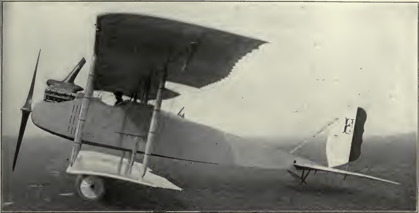
Side view of one of the Farman aeroplanes used for aerial photography.
