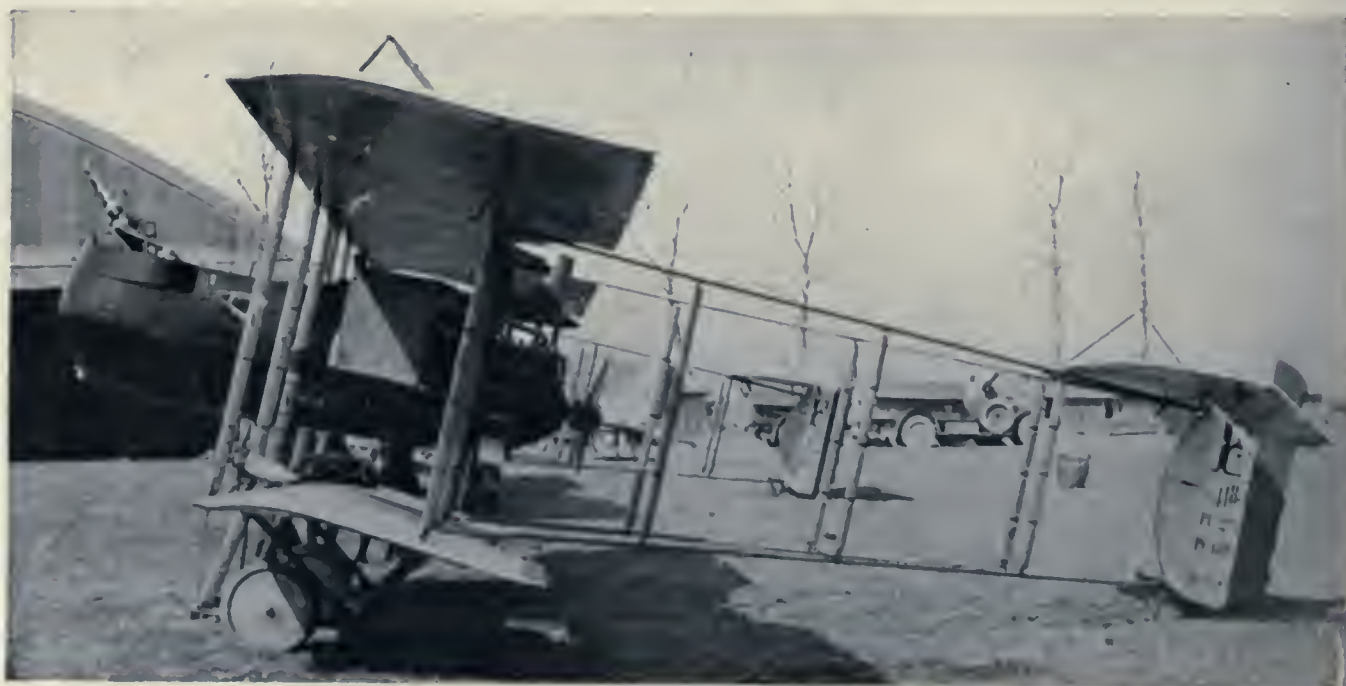
The French Farman machine equipped with a Dietrich motor, used extensively for bombing.
