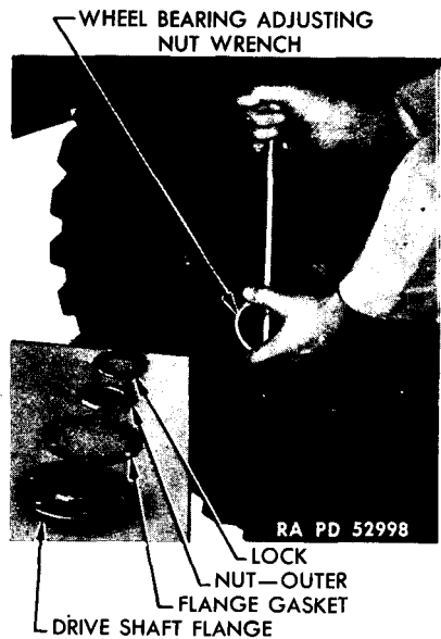
Figure 153—Adjusting Front Wheel Bearing
