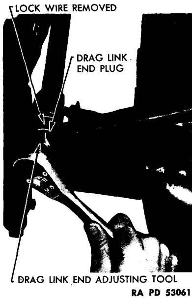
Figure 190—Adjusting Drag Link End
