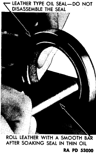
Figure 155—Conditioning Oil Seal
