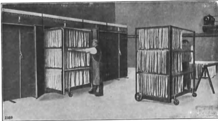
Abb. 42. Trockenschrank (B. Schilde A.-G., Hersfeld H.-N.).
