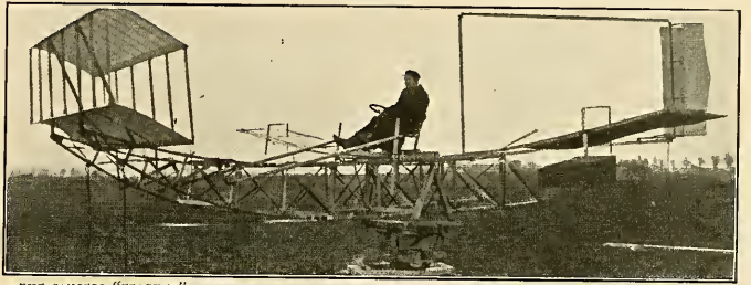
THE SANDERSON "TEACHER"—A DUMMY MACHINE ON A PIVOTED ROCKER TO LEARN FLYING ON TERRA FIRMA.
