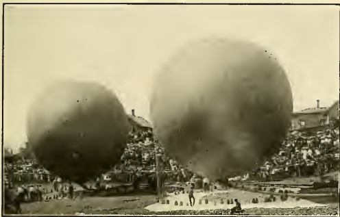
SHOWING POSITION OF SAND-BAGS AND NET AFTER BALLOON IS INFLATED
