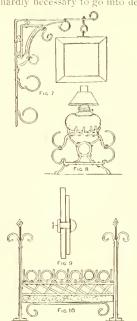
for making these stands, as every part is bent as described in connection with the bending forms, and the portions are simply riveted at the different junctures. Both iron and copper rivets are used as at I, in Fig. 9, a cross sectional view.
