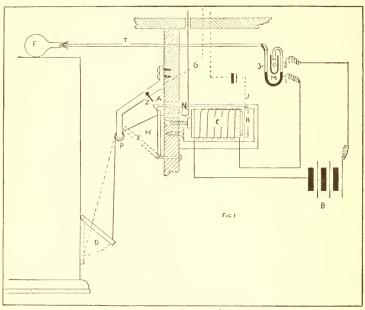
Details of Furnace Regulator Construction
