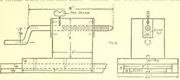
ter, using longer 3.16-in, stove bolts with heads countersunk. Rotate the lathe, and with a gimlet bore a hole at the exact center and through the board. Now take off the board and countersink on the back a place for the head of a coarse threaded screw. Turn in a 13<sub>1</sub>-in, screw, replace the board and any block held on the end of the rotating screw will turn on and be held while being turned.—Contributed by L. L. Winans, Mexico, Mo.
