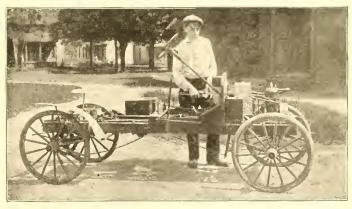
Side View: Seat Removed to Show Construction
