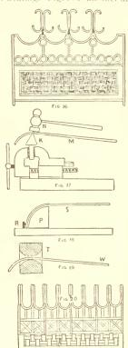
which can be wrought out. The middle adjustment is wire sereen work which may be bought at a hardware store and set into the position shown. Fig. 13 shows a chipping off device useful in connection with this work. Metal chippers can be bought at any tool store. The chipper is placed in the jaws of the vise as at K, and secured there. The strip of metal in process of enttine is marked M. The hammer head is caused to strike the metal just over the cutting edge of the chipper. The quick,
