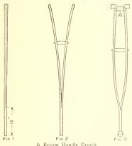
pieces and the handle then riveted as shown in Fig. 2. Another piece was cut as shown at A. Fig. 3, and nailed to the upper ends of each half of the broom handle.—Contributed by Geo. P. Grehore, Nashville, Tenn.
