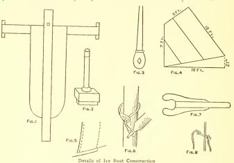
should be serewed to the under side of the 8-ft, plank at the end with the grain running crosswise. Through this bore a hole 1½ in. in diameter in order that the rudder post may fit nicely. The tiller, Fig. 3, should be of hardwood, and about 8 in. long.
