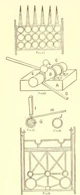
sufficiently stiff by uniting two sides with rivets. The ends at top are looped as shown, while the ends or butts at the base are opened out to make the fect. Rings are shaped on forms and are then riveted to the base cross-piece as illustrated. Crosses are made to describe to central design and the plan is worked out quite readily with the different shapes.
