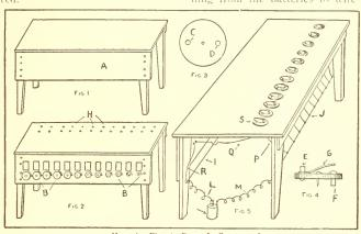
How the Electric Piano Is Constructed
