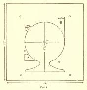
the other piece of wood is an even ½ in, all the way around. Then nail the wheel down firmly, and tack the other piece slightly.
