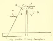
should by all means have a fishing semaphore. This instantly shows from a distance when a fish is on the hook, and any boy
