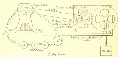
the clockwork and put a weight of about 10 or 12 lb. on the end of the string.
