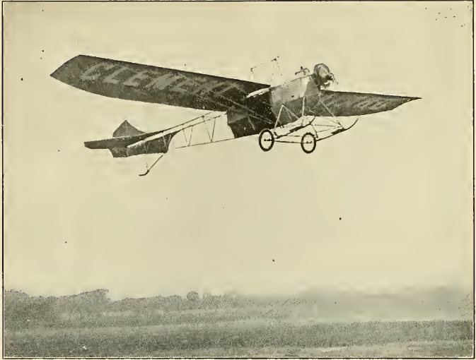
THE CLEMENT-BAYARD MACHINE IN FLIGHT. THIS MACHINE IS FITTED WITH INTER-CHANGEABLE WINGS AND CAN BE FLOWN AS EITHER A MONOPLANE OR A BIPLANE. BELOW WE SHOW IT AS A BIPLANE.
