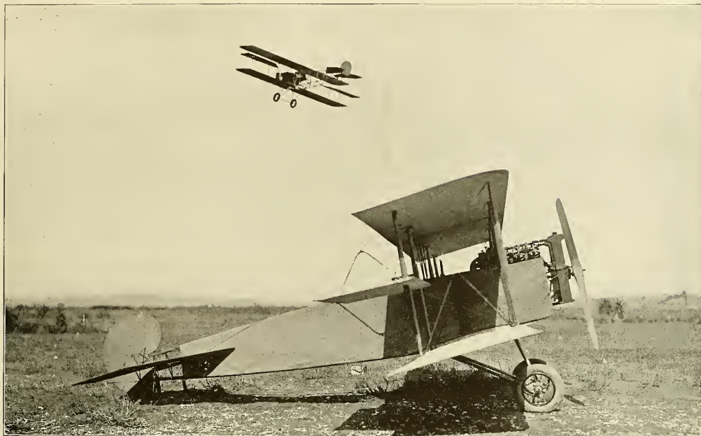
Two views of the new 80 h. p. Curtiss Engine Tractor Biplane, built to the special order of Lincoln Beachey, at the Curtiss factory, at Hammondsport, N. Y. The machine was recently tried out at San Diego, and proved very speedy.
