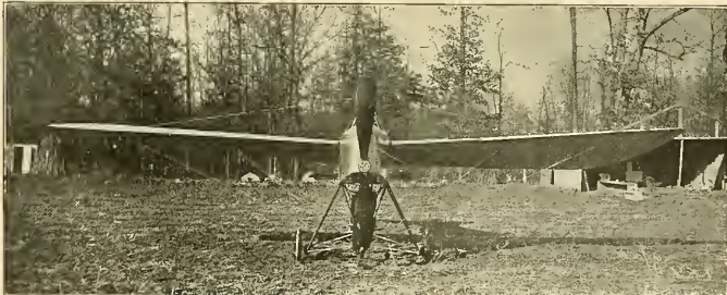
FRONT VIEW OF HEINRICH MONO-BIPLANE SHOWING WARP.
