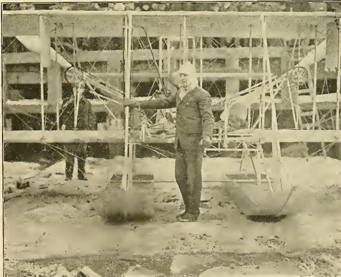
Frank T. Coffyn has been demonstrating lately that winter flying can be made just as popular as summer flying, on condition, of course, that the aviator is dressed warm enough. The above photograph shows him at the bow of his Wright machine, fitted with special rocker pontoons. As can be readily understood the effect of these pontoons is to skim along over the water easily and also over broken ice during the winter in case it is necessary to do so. Mr. Coffyn spent most of the month of February flying about the North and East rivers in juxtaposition to New York City. His flights were of the highly sensational order and were witnessed by hundreds of thousands of people.
