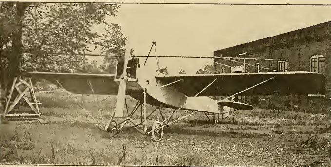
Three-quarter view of the Brooks-Hamilton monoplane, which is designed to be successfully flown with low power and be capable of making extended cross-country trips and rough landings. Note the substantial double wheel and double skid landing chassis and peculiar shaped rattan skid under the rear non-lifting tail.
