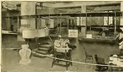
Three-quarter view of the large Farman type hydro-aeroplane designed and built by Paul Schill, of the Max Ams Company, and equipped with an 8-cylinder water-cooled V type 100 H. P. Max Ams motor, which is hand cranked from the seat. A peculiarity of this machine is the way in which the outer sections of the wings slope backward in the form of a large open V.
