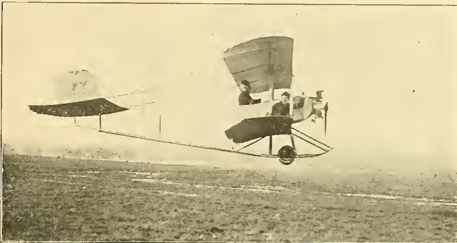
THE SMALL CAUDRON BIPLANE, FITTED WITH ONLY A 30 H. P. 3-CYLINDER Y-TYPE ANZANI, GETTING OFF THE GROUND QUITE EASILY WITH TWO ABOARD. NOTE THE PASSENGER SITTING ON THE PLANE.
