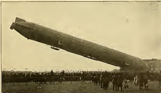
Airship "Deutschland 11." Note steep slant at which Zeppelin passenger airships land. These ships always rise and descend at angles of 13 to 45 degrees.
