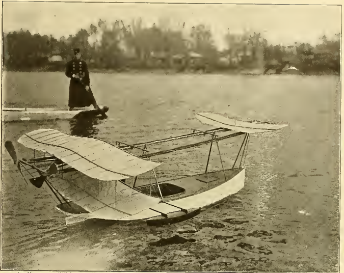
A German "Skimmer," or small one-passenger boat fitted with an aeroplane attachment and driven for short distances by two very powerful rubber band motors. The craft is an experimental one, and is designed for testing the efficiency and stability of various kinds and shapes of planes.
