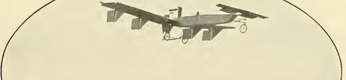
The Latest in Aviation. Professor Reissner flying his novel tail-first monoplane at the Johannisthal field, Germany, in a high wind. Note the peculiar planes with fins and rudders underneath.
