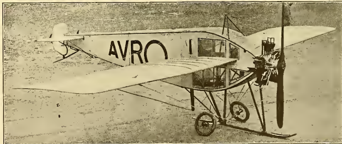
The new enclosed body Avro monoplane. The pilot sits low down inside the fuselage and looks out through the transparent non-inflammable windows. Why the engine has been so placed that it throws oil all over the windows and makes extended flights an impossibility is certainly a mystery. The new Rich enclosed monoplane shown on the next page has the engine placed high up in the fuselage in such a position that the oil is thrown back along the top and not directly onto the windows.
