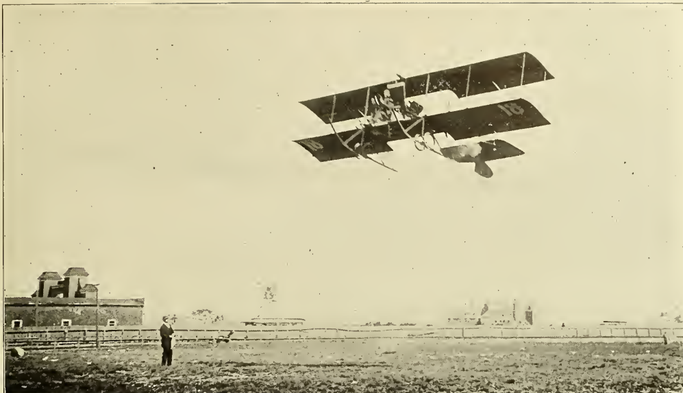
Cecil Peoli, the young Baldwin aviator, flying an 80 H. P. headless Baldwin biplane at Milton, Pa., and making one of his quick rises from a small field. Mr. Peoli states that the quick rising capability of a machine is the main feature of its success for exhibition flying.
