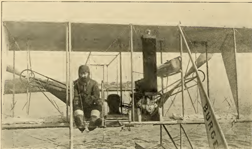
MODEL B-6 INSTALLED IN BURGESS HYDROAEROPLANE
