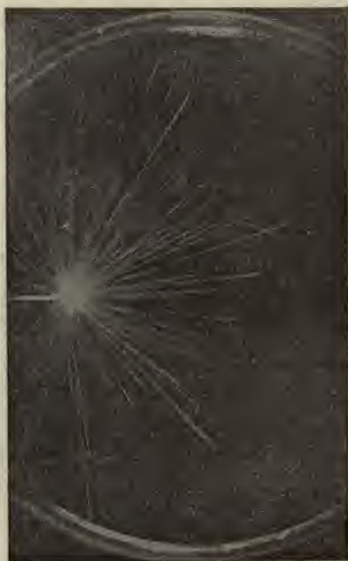
FIG. 19.—Photograph of paths described by \alpha -particles (positive helium ions) emitted from a radioactive substance.
