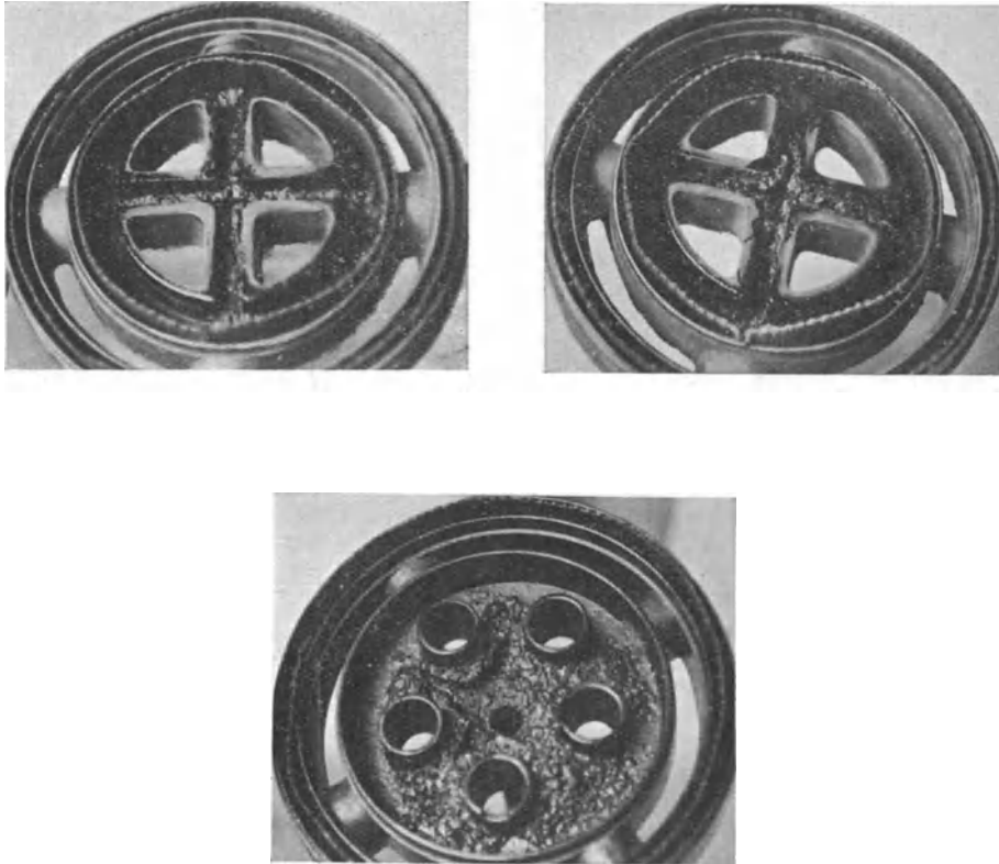
Fig. 258. Carbon formation on range burner bases.
