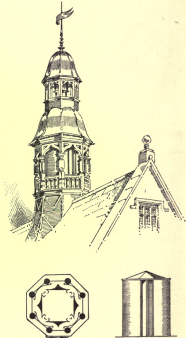
Fig. 592.—Kite's Extract-cowl in Wood Turret.
