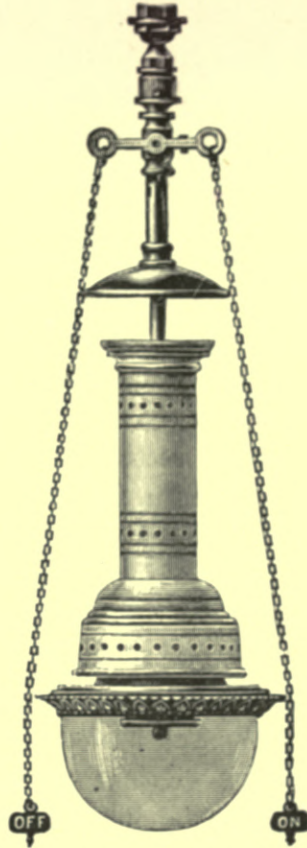
Fig. 651.—Elevation of Wenham Lamp.
