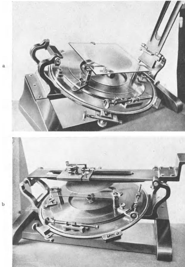
Fig. 4. The Greenwich solar micrometer (open and shut).
