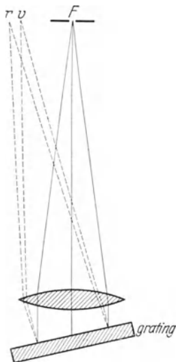
Fig. 15. Diagram of the auto-collimating spectrograph.
