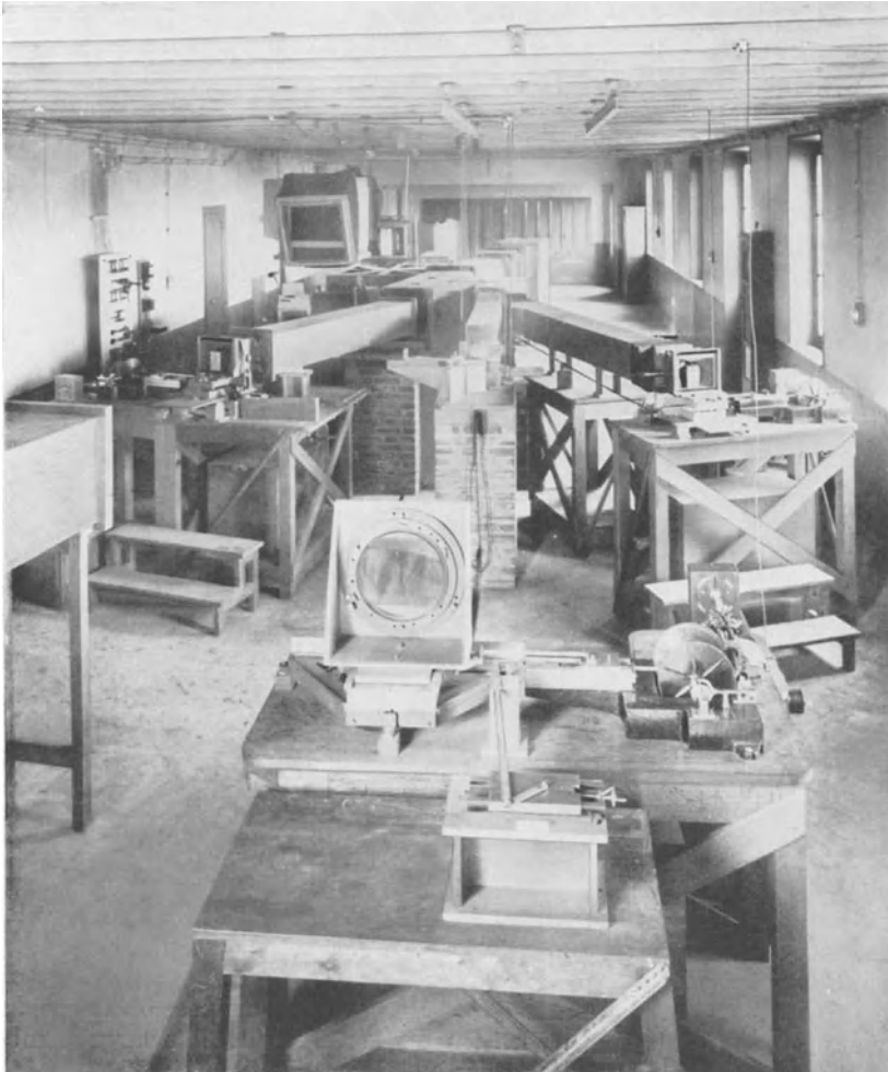
Fig. 23. Quadruple spectroheliograph of the Observatory at Meudon. Four spectroheliographs are combined around the same astronomical objective and collimator. The spectroheliograph of three metres with prisms (left) and the spectroheliograph of three metres (right) are ready for use.
