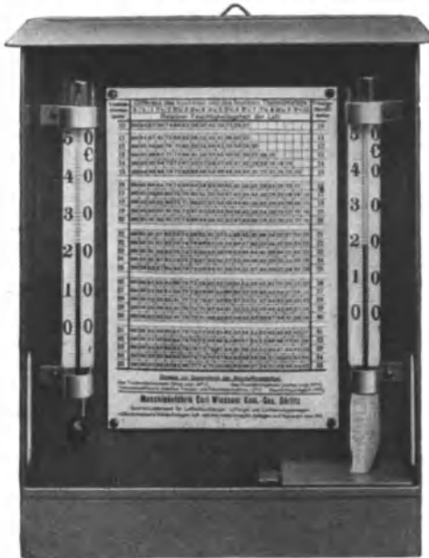
Abb. 21 a. Wandpsychrometer (C. Wießner, Görlitz).
