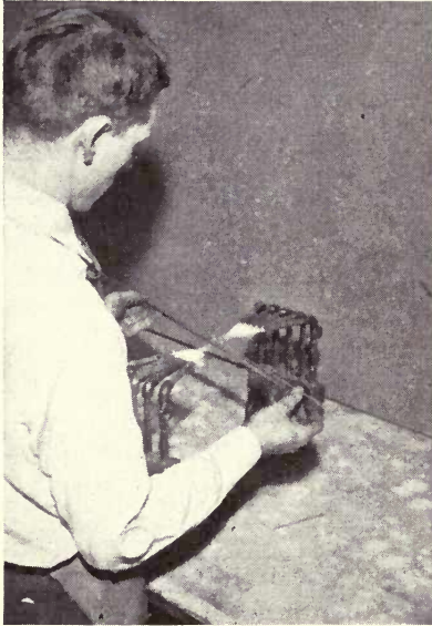
FIG. 42.—Use of cross-fires. Note position of hands.
