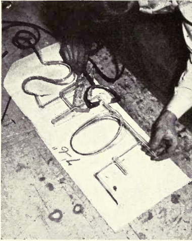
FIG. 53.—Glass blower splicing two letters with hand torch over asbestos layout.
