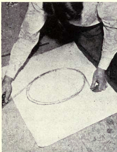
FIG. 55.—Matching a curved (ribbon-fire) bend to a layout.
