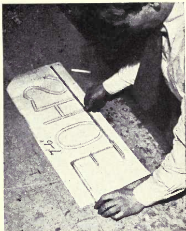
FIG. 54.—Matching letter to asbestos layout.
