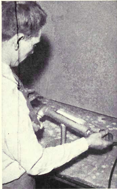
FIG. 43.—Use of ribbon fire. Note method of holding glass as it is rotated in flame.
