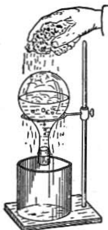
FIG. 232.—Boiling at reduced pressure.
