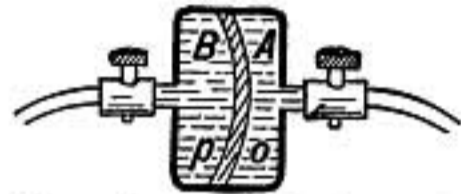
FIG. 316. — Hydraulic model of Leyden jar.
