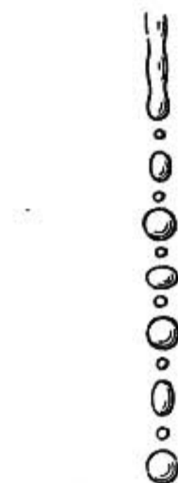
FIG. 152.—Jet breaking into drops.
