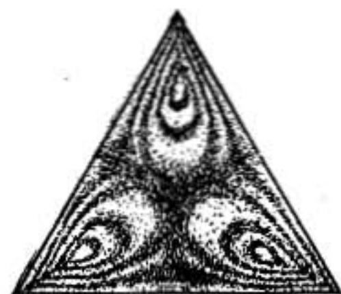
FIG. 608.—Strain figure in a triangle of tempered glass by polarized light.
