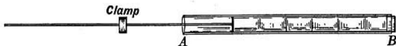
FIG. 191.—Kundt's tube experiment.
