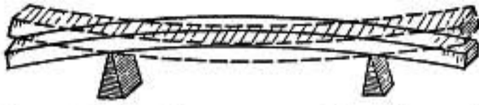
FIG. 197.—Transverse vibration of rod.
