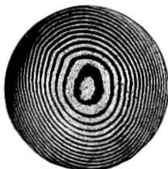
FIG. 572.—Newton's rings in sodium light.
