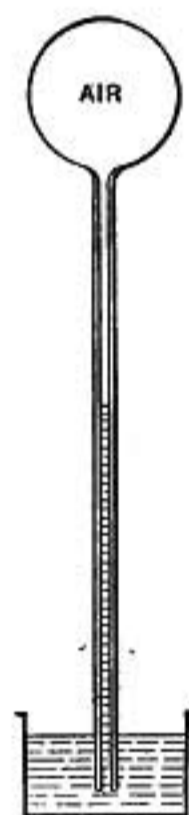
FIG. 206. Galileo's air thermometer.
