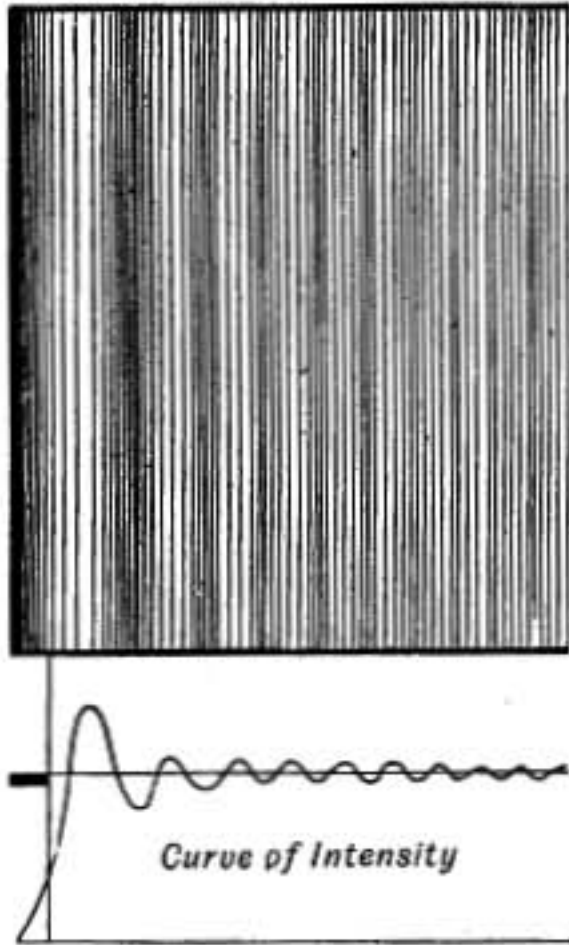
FIG. 575.—Diffraction bands at the edge of a shadow. The vertical line is edge of the geometrical shadow.
