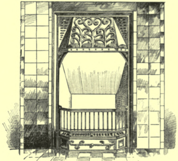
Fig. 475.—Front View of Shorland's Fireplace.
