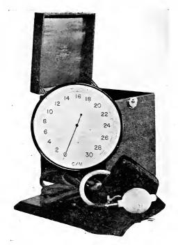
Fig. 34.—Sphygmomanometer with a dial 8 inches in diameter and may be read across a room. This large dial magnifies the oscillations of the needle. The range is 300 mm. The dial is adjustable to any position.
