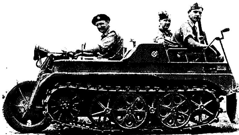
Figure 5. —Captured German half-track vehicle ( Kettenkrad ) frequently used for transport by mountain troops.
