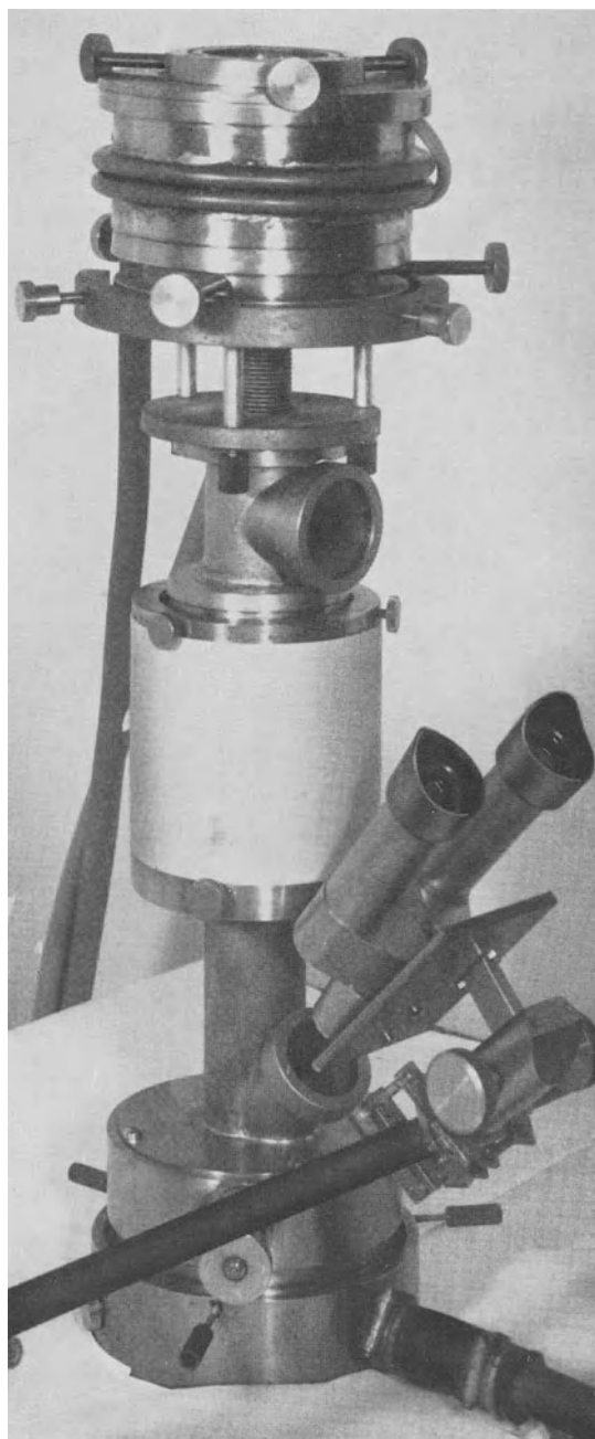
Fig. 13. The Delft X-ray projection microscope, constructed early in 1957. Binocular observation of the focusing screen. In its present form the tilting is omitted and a 30\times monocular microscope is used for focusing (cf. fig. 12).
