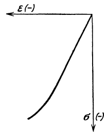
Abb. 9. \sigma = f(\epsilon) Druck.
