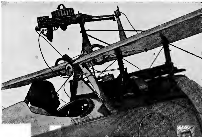
Machine Gun mounted to Fire over the Blades of the Propeller
