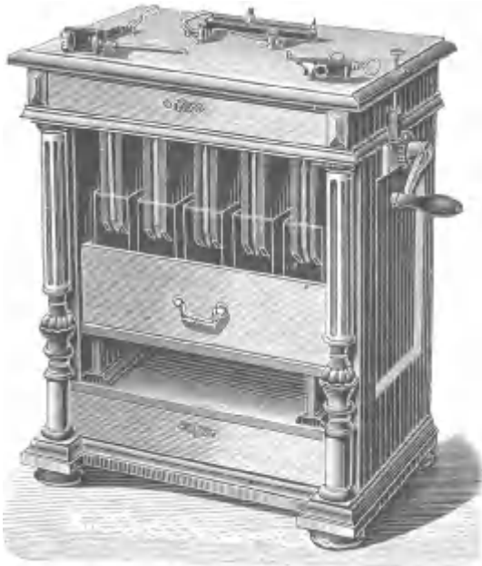
Fig. 65. —10-CELL BICHRIMATE BATTERY.—This battery is suitable for all electric lighting and cautery purposes; but being a stationary apparatus, it is most suitable for hospitals or the consulting-room. Owing to the large surface of the plates and the capacity of the cells, there is ample reserve of power, and the solution will last from 6 to 12 months, when in constant use, without recharging. The rack action at the side allows of the plates being immersed only to the required depth. The cells should be entirely lowered when the battery is out of use. The apparatus is fitted with a rheostat, by which a certain amount of resistance is introduced into the circuit, and can be gradually reduced to the required point suitable for the various cautery points and lighting apparatus.
