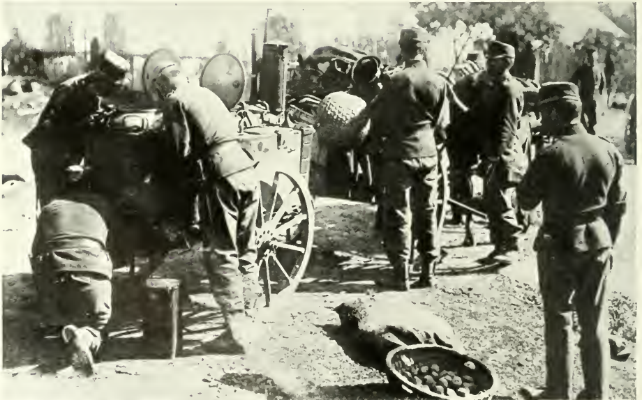
Portable cooking stoves, used in the Austrian Army, which enable cooking to be done while the troops march.
