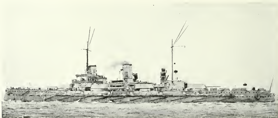
German battleship Nassau , 18,600 tons, carrying a main armament of twelve 11-inch guns.
