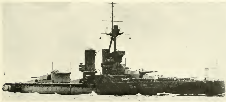
British battleship Iron Duke , 25,000 tons, carrying a main armament of ten 13.5-inch guns.
