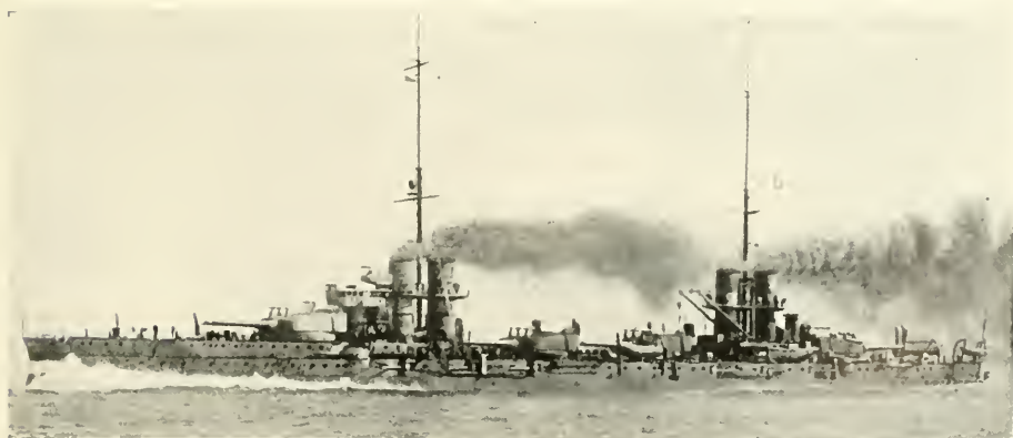
Italian battleship Dante Alighieri , 19,400 tons, carrying a main armament of twelve 12-inch guns.
