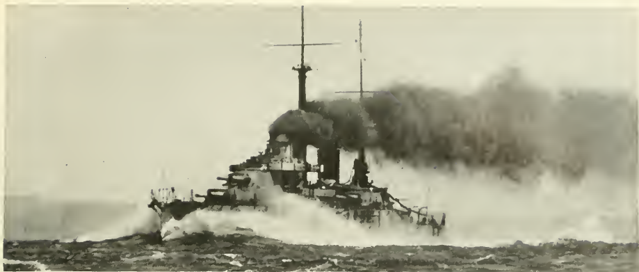
French battleship Paris , 23,000 tons, carrying a main armament of twelve 12-inch guns.
