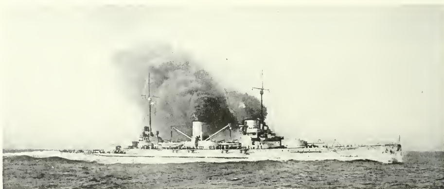
German battle-cruiser Moltke , 22,640 tons, carrying a main armament of ten 11-inch guns.
