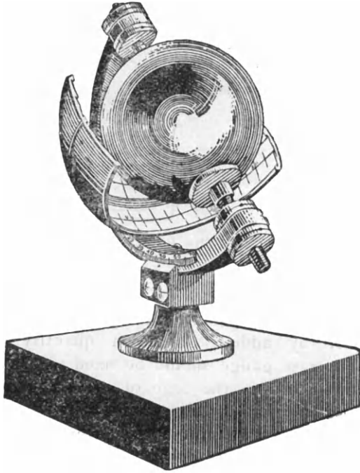
Fig. 16—The Sunshine Recorder.
