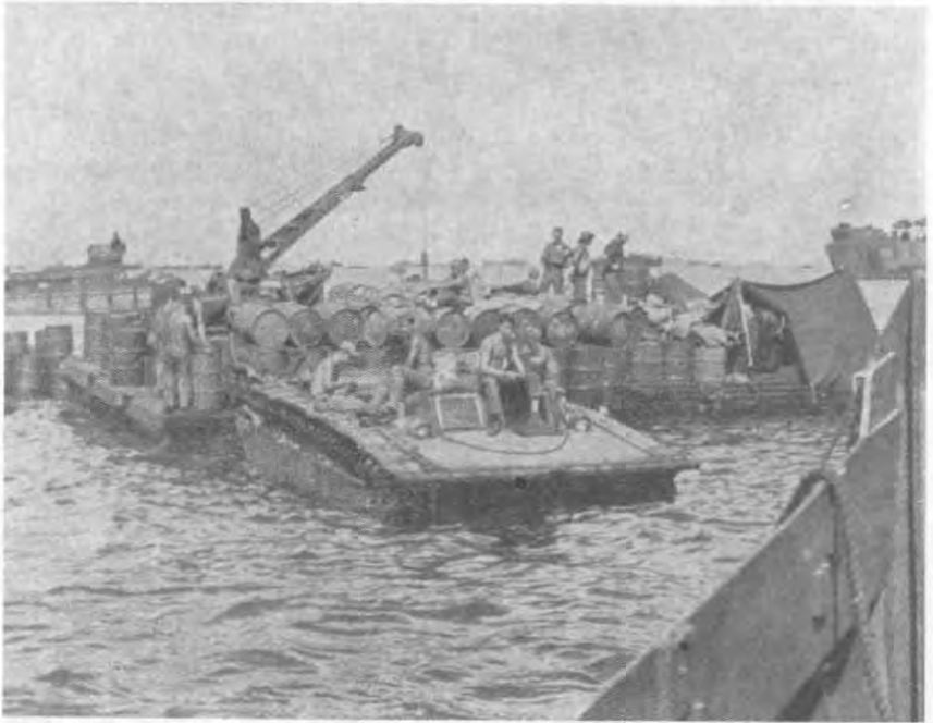
CRANES AT REEF'S EDGE transferred supplies from landing craft to LVT's and dukws which could cross reef at any time regardless of the tide. The barge, being used as a platform for crane in this photograph, is preparing to load fuel on an Alligator. (Photo taken W + 4)
