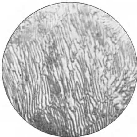
Abb. 21 v = 1650 Perlit (0,9% Kohlenstoff).
