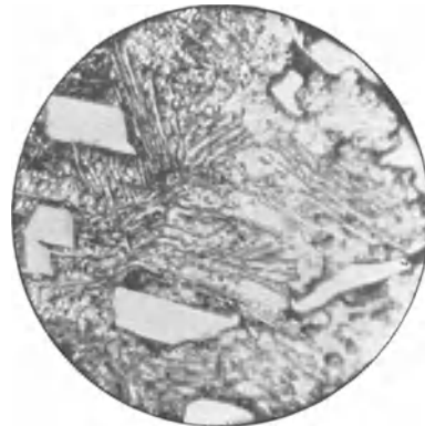
Abb. 22 v = 900 Zementit und Perlit (1,3% Kohlenstoff).
