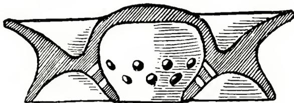
FIG. 231. SECTION OF CLAY 'FIRE-BOX'.
