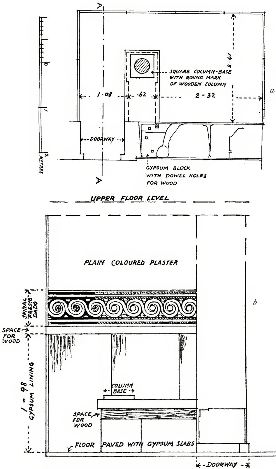
FIG. 253. PLAN AND ELEVATION OF BATH-ROOM (THEODORE FYFE).
