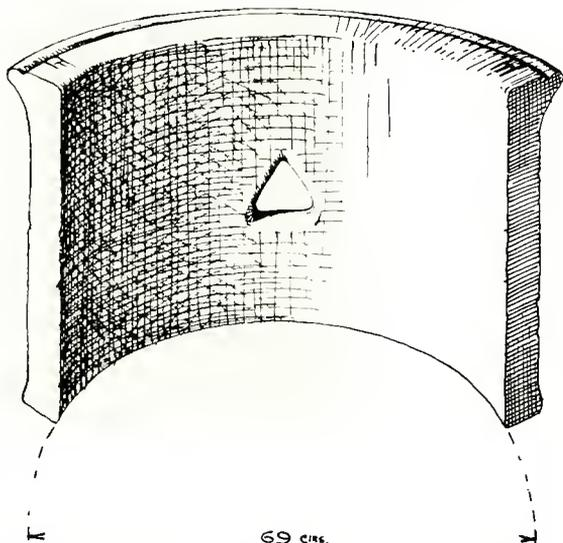
FIG. 175. SECTION OF TERRA-COTTA DRUM OF WELL.
