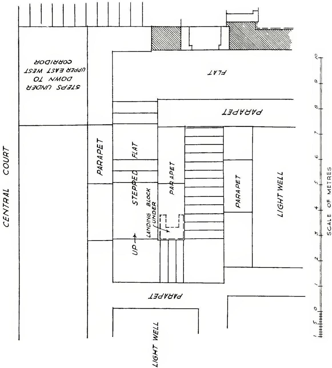
FIG. 337. PLAN OF UPPERMOST SYSTEM OF GRAND STAIRCASE, SHOWING STEPPED ASCENT TO ROOF-FLAT: CHRISTIAN C. T. DOLL.
