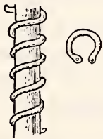
FIG. 1. Probable method of making links for mail.
