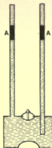
Fig. 174. — Boiler, with Pipes frozen at A A.
