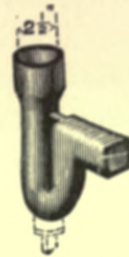
Fig. 194.—View of 1\frac{1}{4} -inch Anti-D Trap, with enlarged Mouth.
