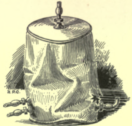
Fig. 177.—View of a Collapsed Cylinder.
