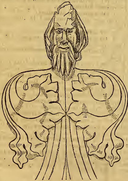
FINIAL FROM WELLS CHURCH, NORFOLK. terminities or finishing point or pinnacles in Gothic architecture. Sometimes used for the pinnacle itself.
