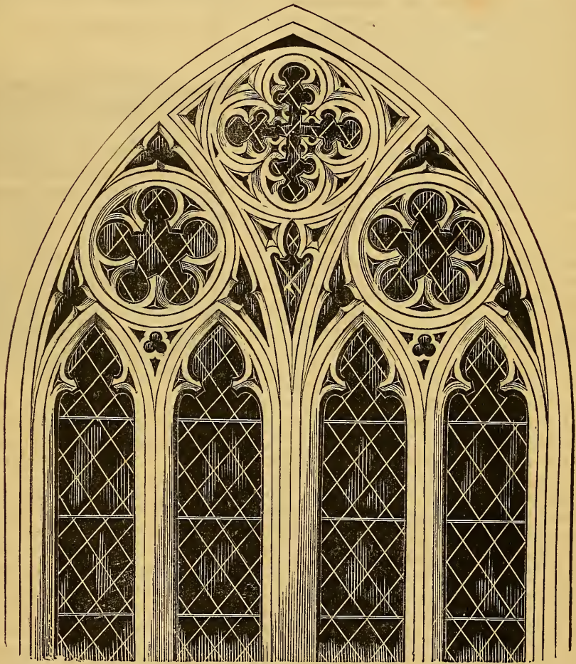
DESIGN FOR TRACERY FOR A GOTHIC WINDOW.
