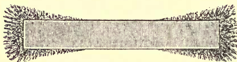
FIG. 64. DISTRIBUTION OF IRON FILINGS ON A STRAIGHT BAR MAGNET
