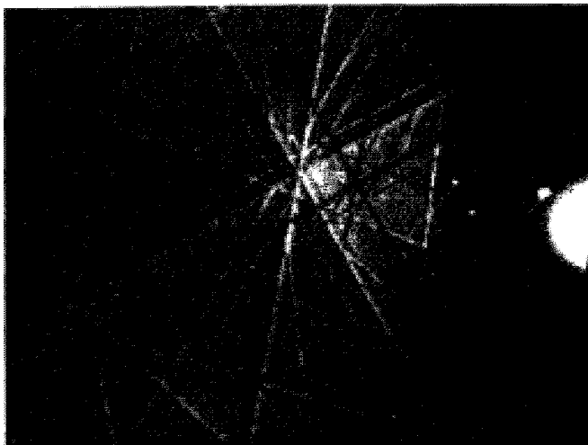
Fig. 41. Reflection from a rocksalt face cut in an arbitrary direction and lightly etched.
