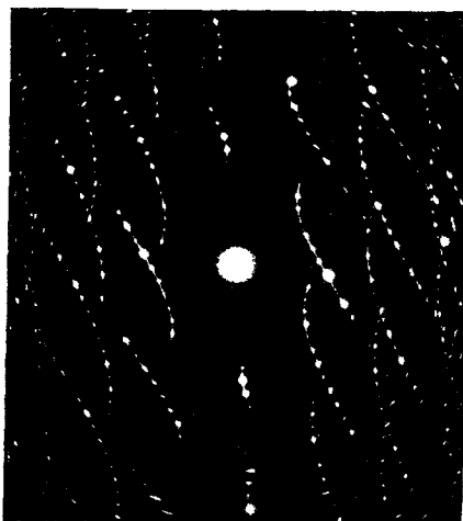
Fig. 20. Rotation-transmission pattern from very thin undistorted molybdenite flake inclined at 70^\circ to axis of rotation.
