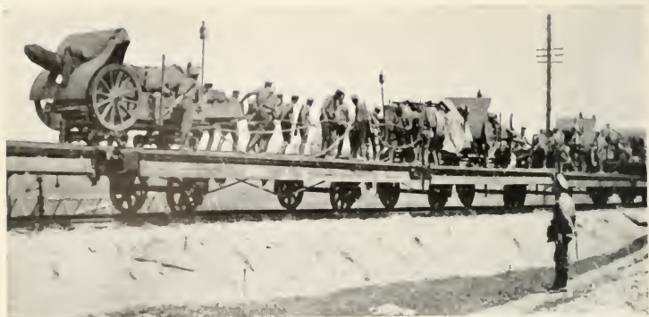
Transport of Russian artillery. By means of small trucks running on rails laid on flat cars the handling of guns by rail-way is greatly expedited.
