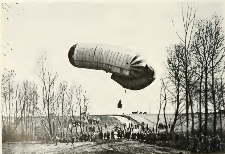
French observation balloon about to arise. The observer is in the "nacelle," or basket, suspended underneath and communicates with the ground by telephone. The large semicircular curved bag at the rear is open at the front to allow the wind to fill it and thus hold the balloon's head to the wind. A gasoline windlass on a truck hauls the balloon back to the ground when desired.
