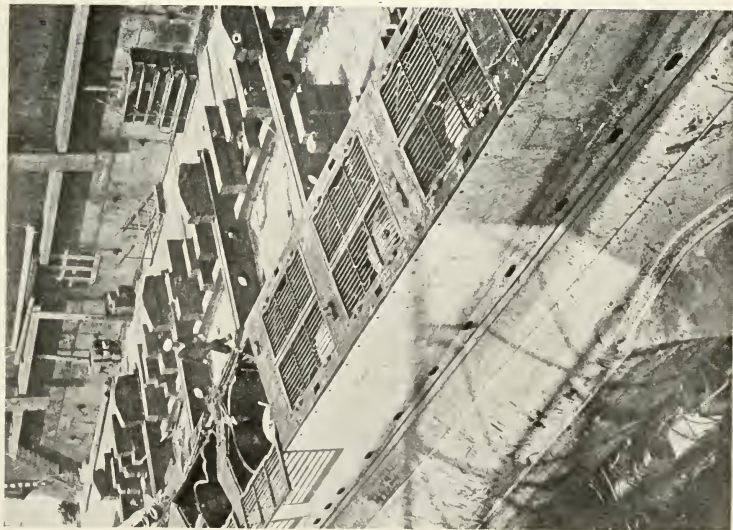
Mine-laying German submarine captured by the British. The mines with their anchors are in the grating-covered compartments. Their release is controlled from the conning tower.
