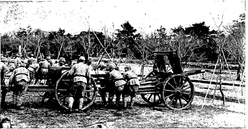
Figure 52. Assembly of Model 4 (1915) 150-mm howitzer: Connecting rear trail section to carriage.
