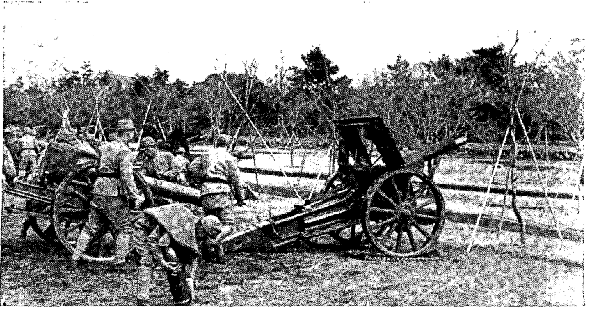
Figure 51. Assembly of Model 4 (1915) 150-mm howitzer: bringing up the tube and rear trail section.
