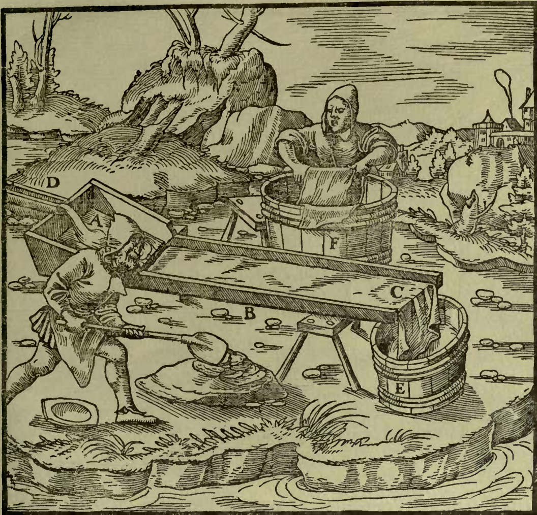
A—HEAD OF FRAME. B—FRAME. C—CLOTH. D—SMALL LAUNDER. E—TUB SET BELOW THE FRAME. F—TUB IN WHICH CLOTH IS WASHED.
