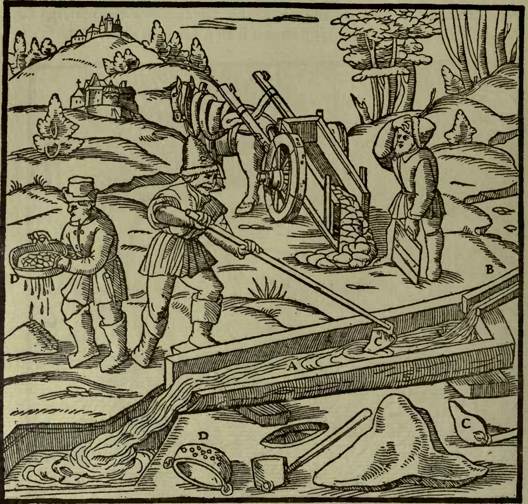
A—TROUGH. B—LAUNDER. C—HOE. D—SIEVE.
