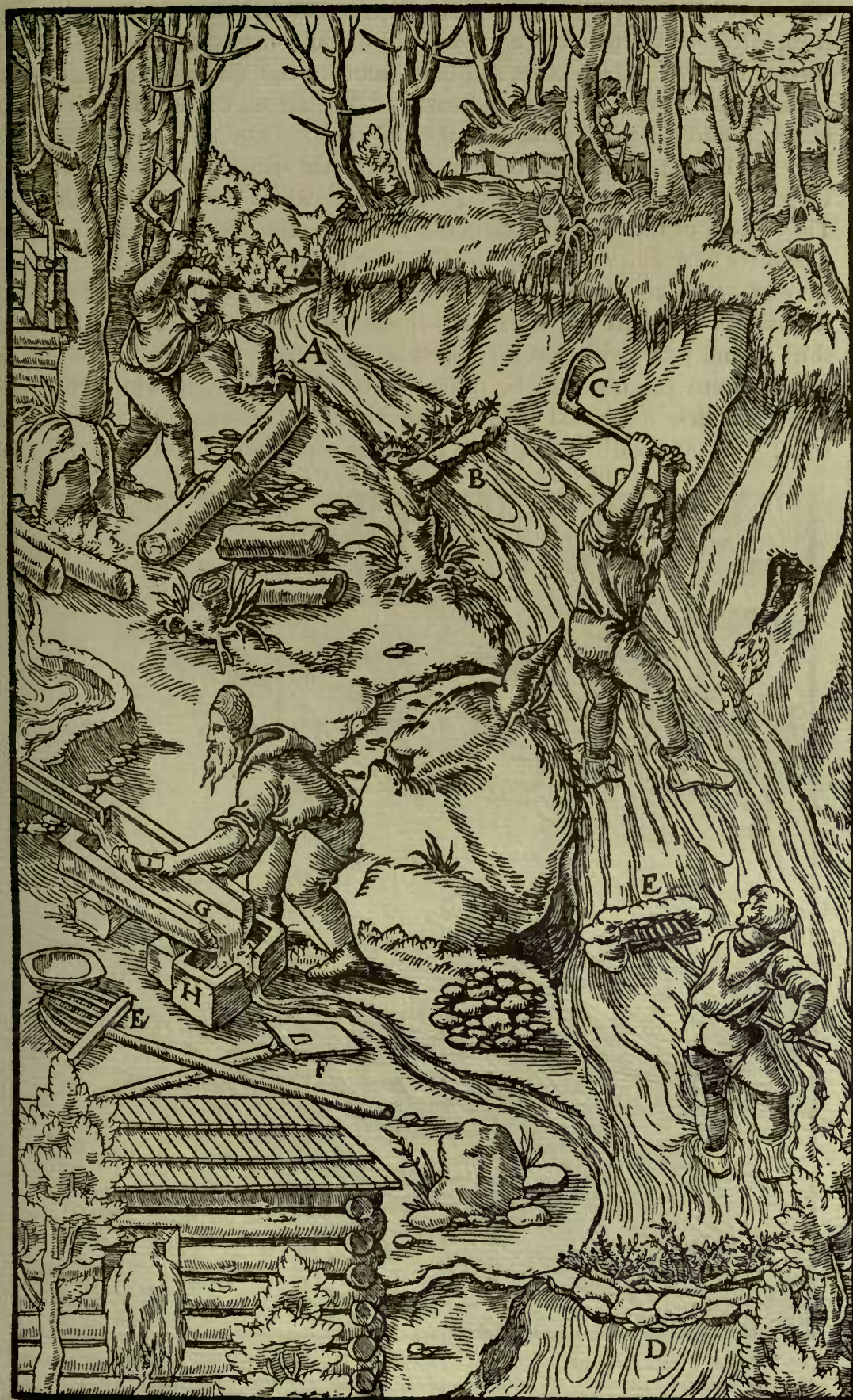
A—STREAM. B—DITCH. C—MATTOCK. D—PIECES OF TURF. E—SEVEN-PRONGED FORK. F—IRON SHOVEL. G—TROUGH. H—ANOTHER TROUGH BELOW IT. I—SMALL WOODEN TROWEL.
