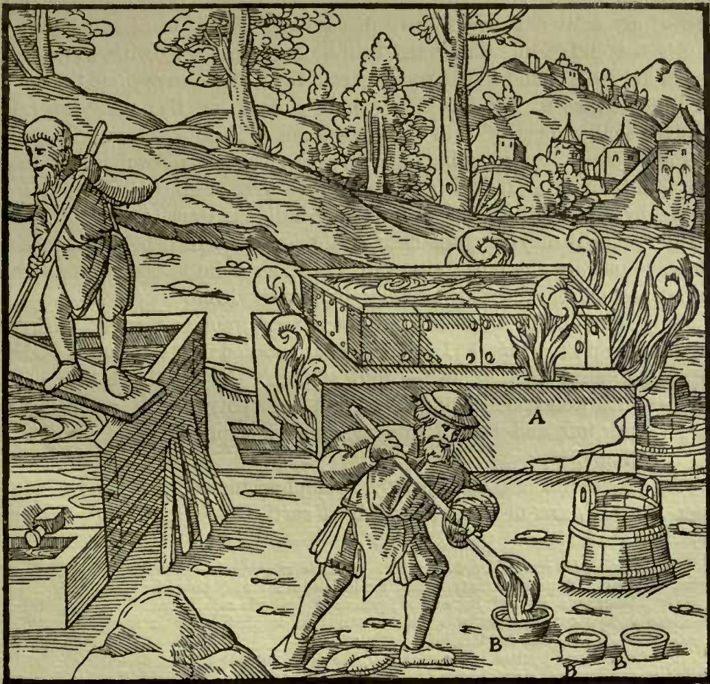
A—CALDRON. B—MOULDS. C—CAKES.
