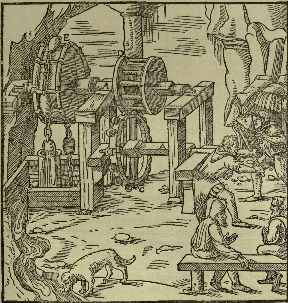
A—AXLES. B—LEVERS. C—TOOTHED DRUM. D—DRUM MADE OF RUNDLES. E—DRUM IN WHICH IRON CLAMPS ARE FIXED.
