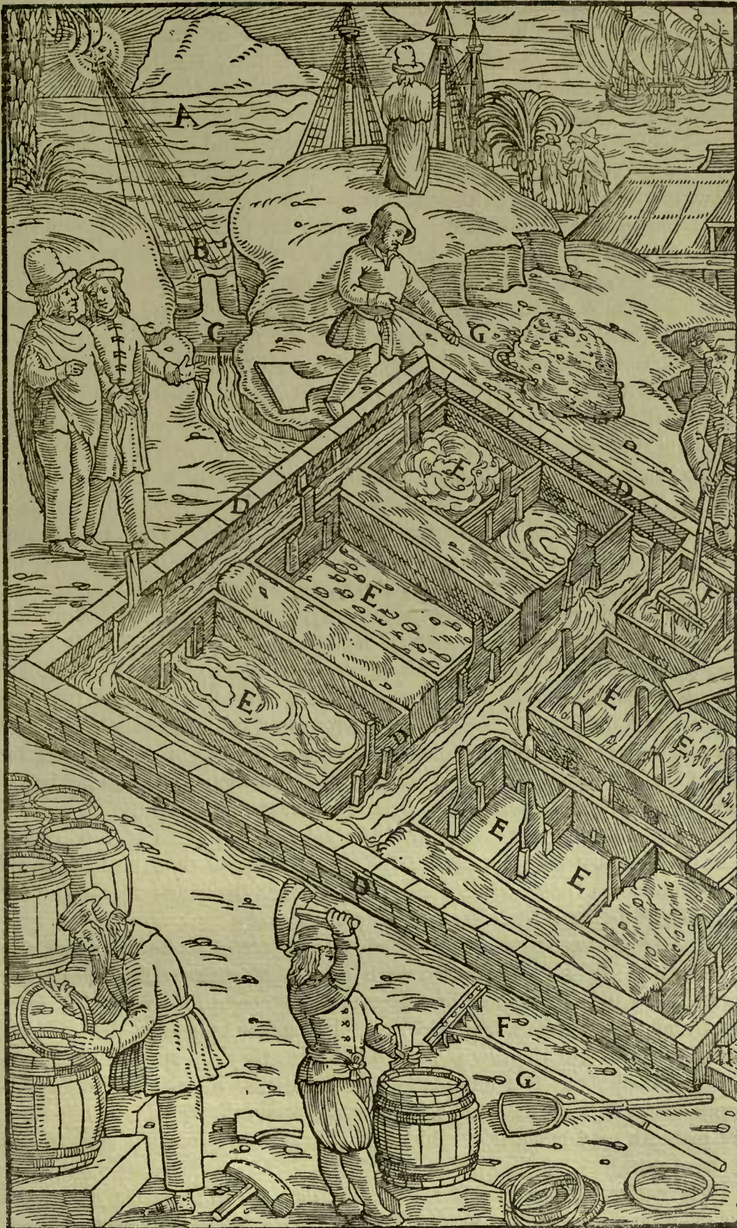
A—SEA. B—POOL. C—GATE. D—TRENCHES. E—SALT BASINS. F—RAKE. G—SHOVEL.
