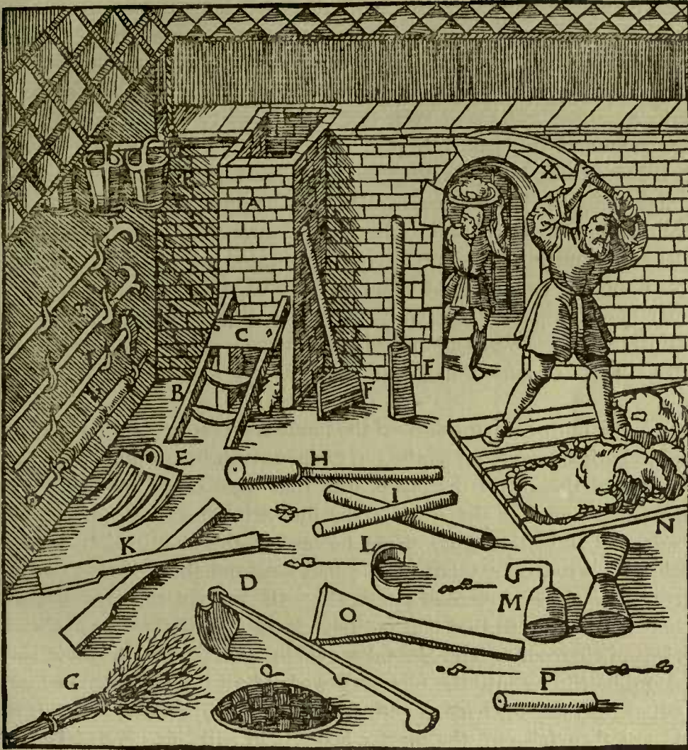
A—FURNACE. B—LADDER. C—BOARD FIXED TO IT. D—HOE. E—FIVE-TOOTHED RAKE. F—WOODEN SPATULA. G—BROOM. H—RAMMER. I—RAMMER, SAME DIAMETER. K—TWO WOODEN SPATULAS. L—CURVED BLADE. M—BRONZE RAMMER. N—ANOTHER BRONZE RAMMER. O—WIDE SPATULA. P—ROD. Q—WICKER BASKET. R—TWO BUCKETS OF LEATHER IN WHICH WATER IS CARRIED FOR PUTTING OUT A CONFLAGRATION, SHOULD THE officina CATCH FIRE. S—BRASS PUMP WITH WHICH THE WATER IS SQUIRTED OUT. T—TWO HOOKS. V—RAKE. X—WORKMAN BEATING THE CLAY WITH AN IRON IMPLEMENT.
