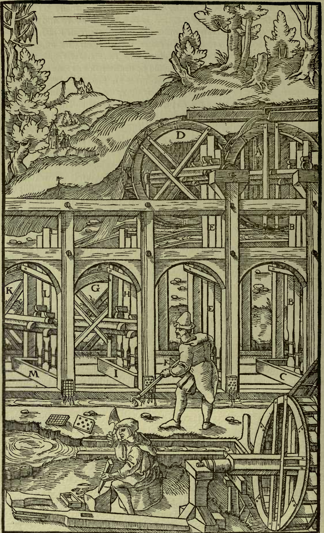
A—FIRST MACHINE. B—ITS STAMPS. C—ITS MORTAR-BOX. D—SECOND MACHINE. E—ITS STAMPS. F—ITS MORTAR-BOX. G—THIRD MACHINE. H—ITS STAMPS. I—ITS MORTAR-BOX. K—FOURTH MACHINE. L—ITS STAMPS. M—ITS MORTAR-BOX.
