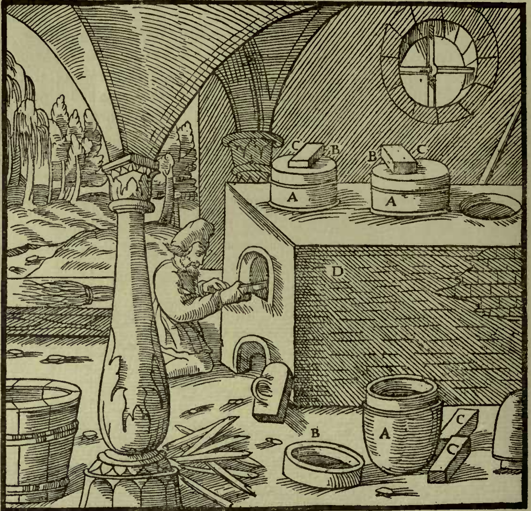
A—POTS. B—LIDS. C—STONES. D—FURNACE.
