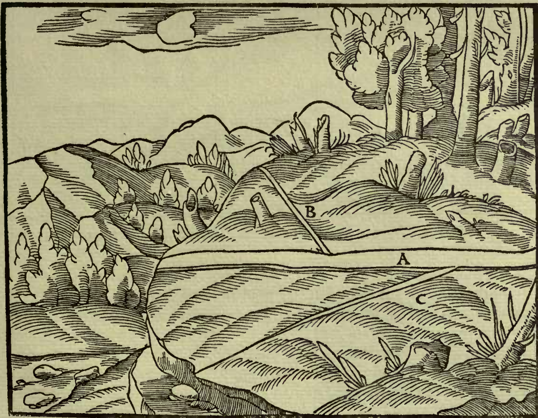
A—VEIN. B— Fibra incumbens FROM THE SURFACE OF THE HANGINGWALL. C—SAME FROM THE FOOTWALL.
