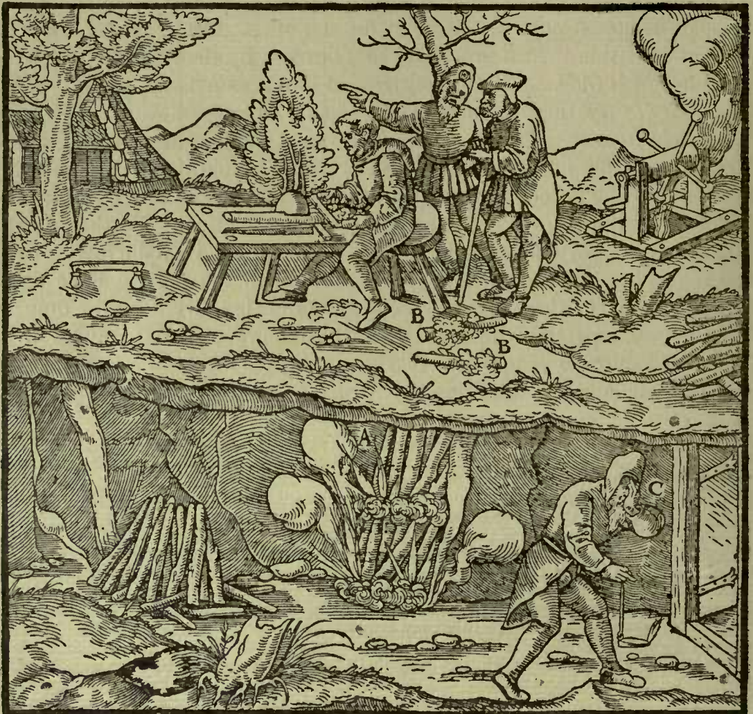
A—KINDLED LOGS. B—STICKS SHAVED DOWN FAN-SHAPED. C—TUNNEL.
