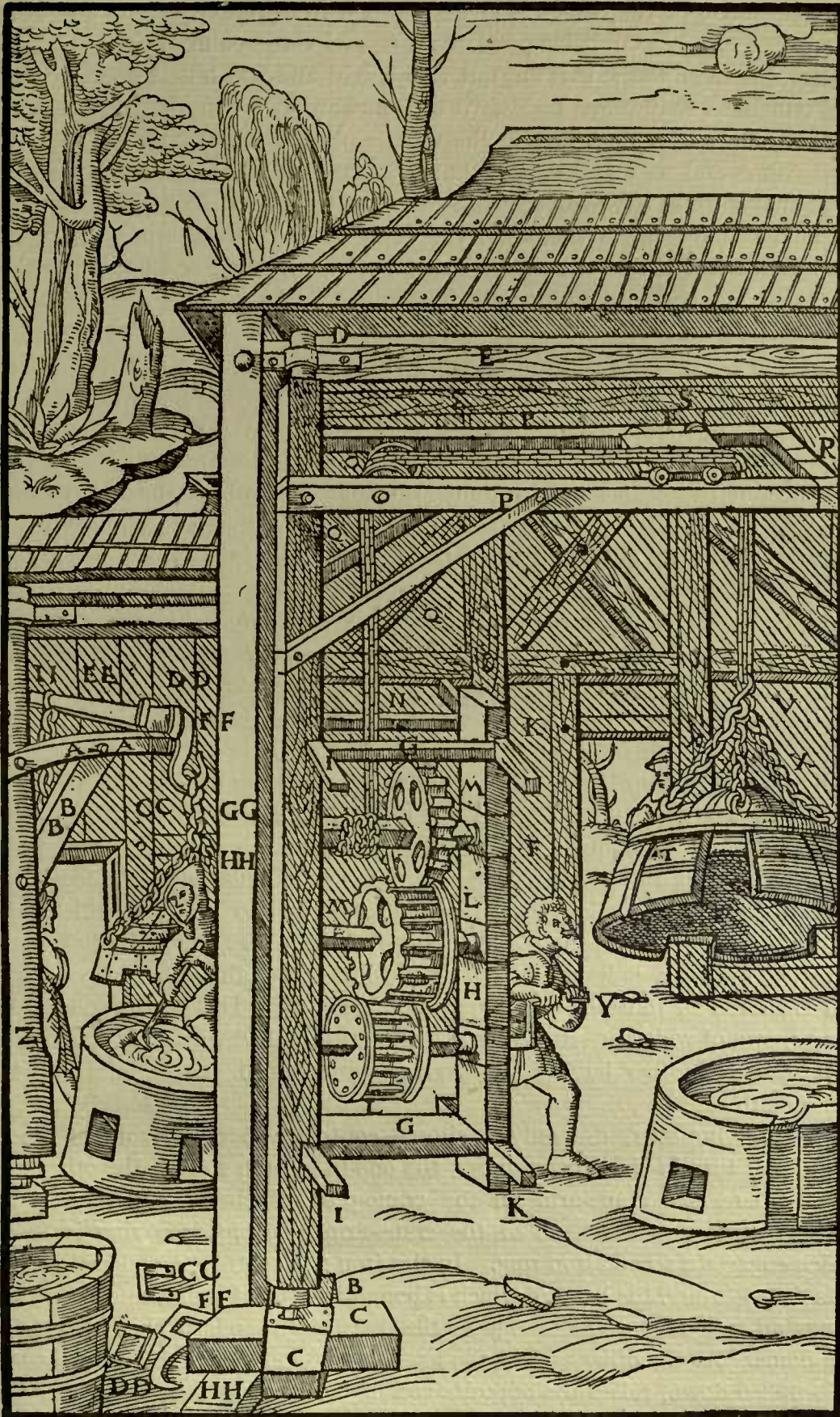
A—CRANE-POST. B—SOCKET. C—OAK CROSS-SILLS. D—BAND. E—ROOF-BEAM. F—FRAME. G—LOWER SMALL CROSS-BEAM. H—UPRIGHT TIMBER. I—BARS WHICH COME FROM THE SIDES OF THE CRANE-POST. K—BARS WHICH COME FROM THE SIDES OF THE UPRIGHT TIMBER. L—RUNDLE DRUMS. M—TOOTHED WHEELS. N—CHAIN. O—PULLEY. P—BEAMS OF THE CRANE-ARM. Q—OBLIQUE BEAMS SUPPORTING THE BEAMS OF THE CRANE-ARM. R—RECTANGULAR IRON PLATES. S—TROLLEY. T—DOME OF THE FURNACE. V—RING. X—THREE CHAINS. Y—CRANK. Z—THE CRANE-POST OF THE OTHER CONTRIVANCE. AA—CRANE-ARM. BB—OBLIQUE BEAM. CC—RING OF THE CRANE-ARM. DD—THE SECOND RING. EE—LEVER-BAR. FF—THIRD RING. GG—HOOK. HH—CHAIN OF THE DOME. II—CHAIN OF THE LEVER-BAR
