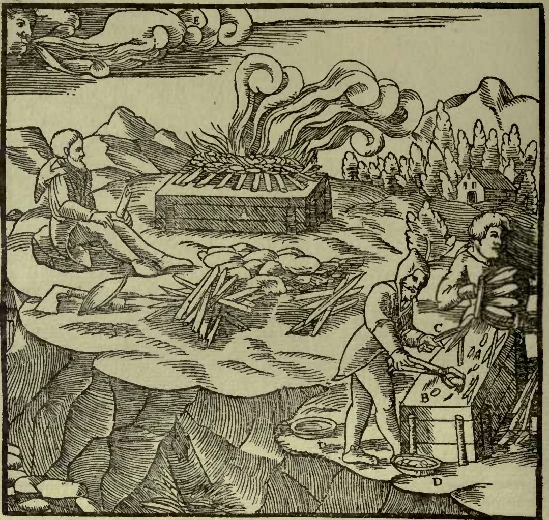
A—HEARTH IN WHICH ORE IS MELTED. B—HEARTH ON WHICH LIE DROPS OF BISMUTH. C—TONGS. D—BASKET. E—WIND.
