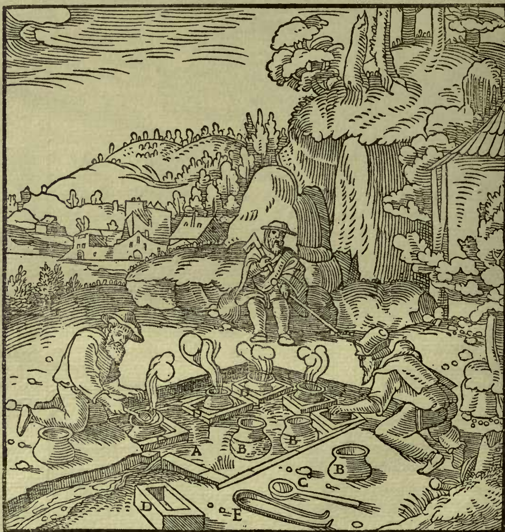
A—POOL. B—POTS. C—LADLE. D—PANS. E—TONGS.
