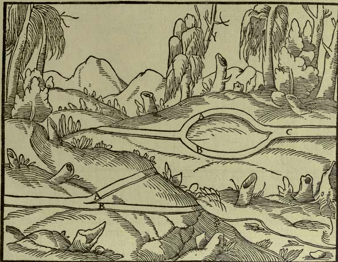
A, B—VEINS DIVIDING. C—THE SAME JOINING.
