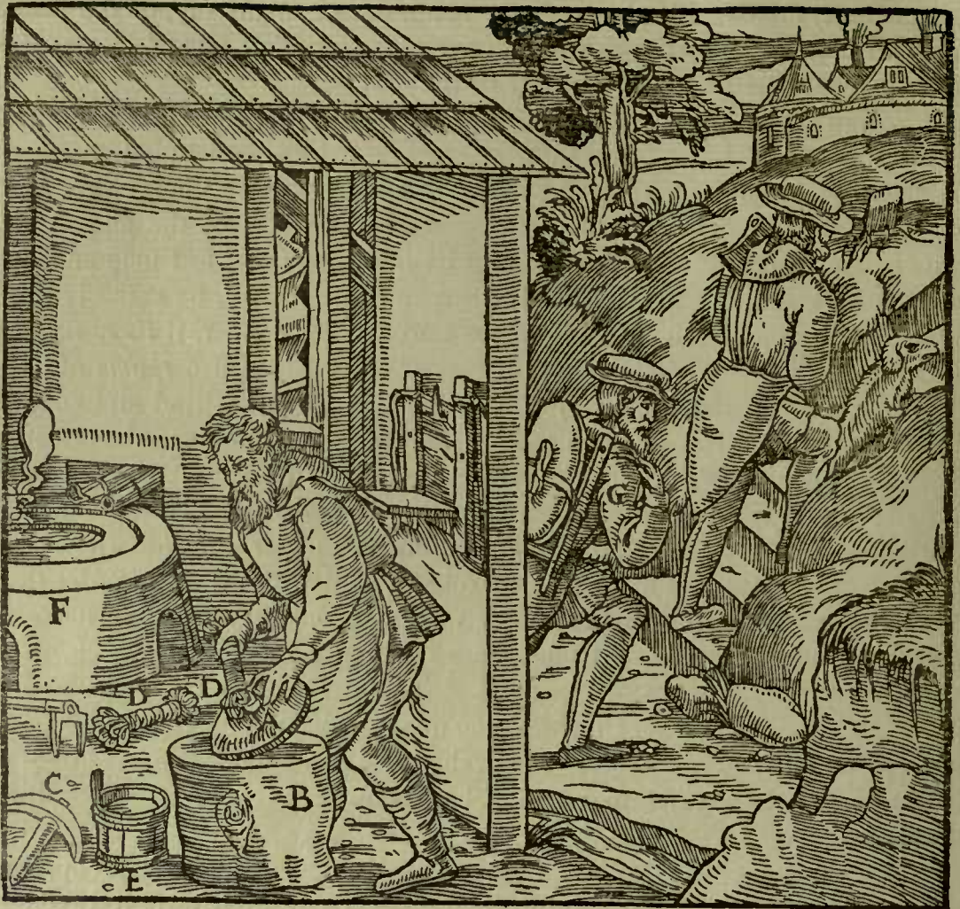
A—CAKE. B—STONE. C—HAMMER. D—BRASS WIRE. E—BUCKET CONTAINING WATER. F—FURNACE FROM WHICH THE CAKE HAS BEEN TAKEN, WHICH IS STILL SMÖKING. G—LABOURER CARRYING A CAKE OUT OF THE WORKS.
