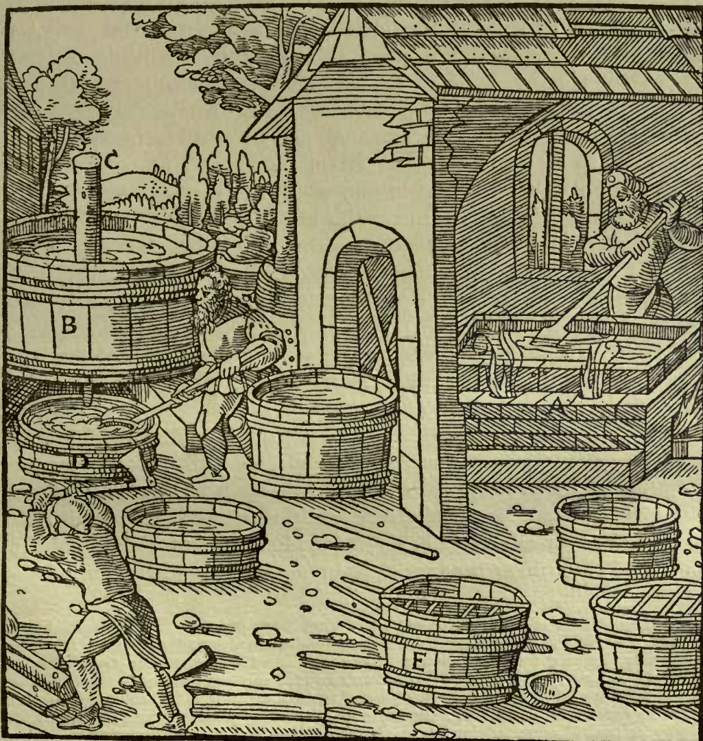
A—CALDRON. B—LARGE VAT INTO WHICH SAND IS THROWN. C—PLUG. D—TUB. E—VAT CONTAINING THE RODS.
