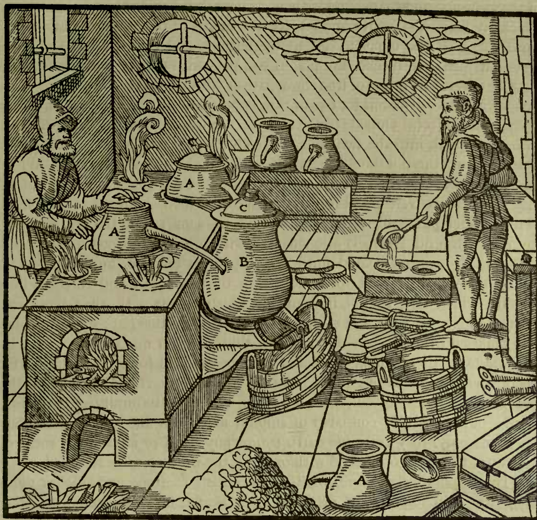
A—POTS HAVING SPOUTS. B—POTS WITHOUT SPOUTS. C—LIDS.
