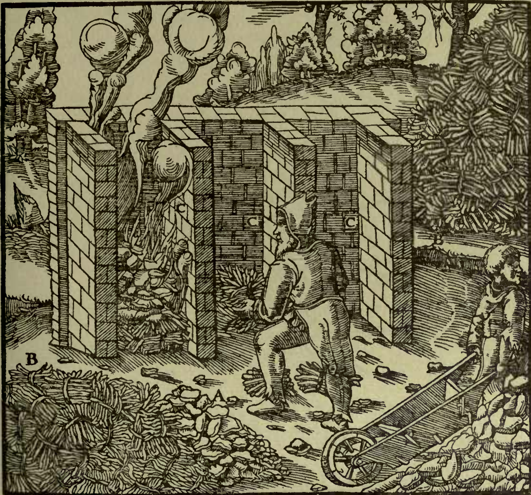
A—CAKES. B—BUNDLES OF FAGGOTS. C—FURNACES.
