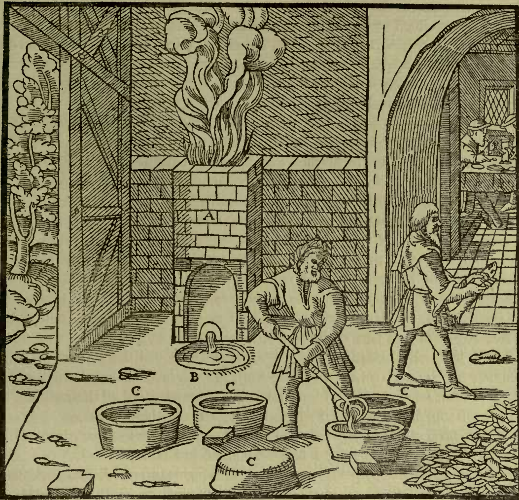
A—FURNACE. B—FOREHEARTH. C—OBLONG MOULDS.
