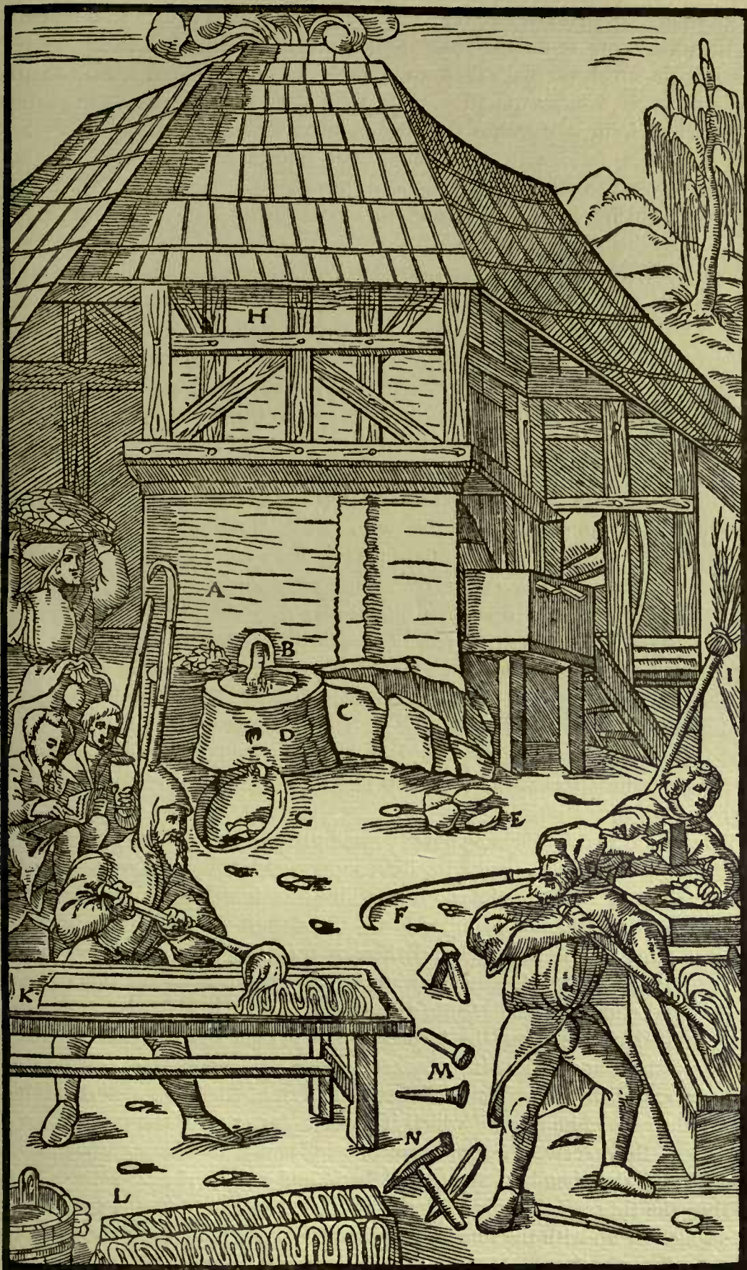
A—FURNACE. B—ITS TAP-HOLE. C—FOREHEARTH. D—ITS TAP-HOLE. E—SLAGS. F—SCRAPER. G—DIPPING-POT. H—WALLS OF THE CHIMNEY. I—BROOM. K—COPPER PLATE. L—LATTICEWORK BARS. M—IRON SEAL OR DIE. N—HAMMER.
