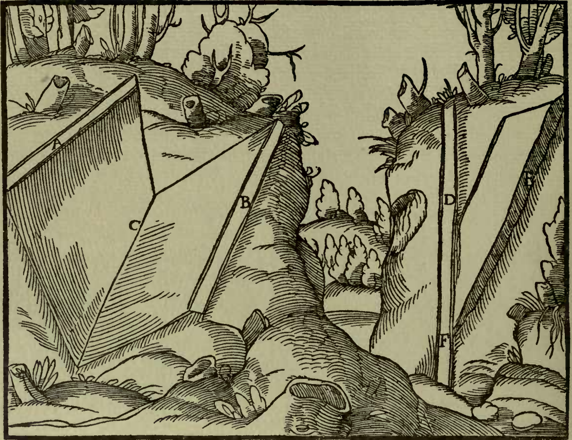
A, B—Two veins descend inclined and dip toward each other. C—JUNCTION. Likewise two veins. D—INDICATES ONE DESCENDING VERTICALLY. E—MARKS THE OTHER DESCENDING INCLINED, WHICH DIPS TOWARD D. F—THEIR JUNCTION.
