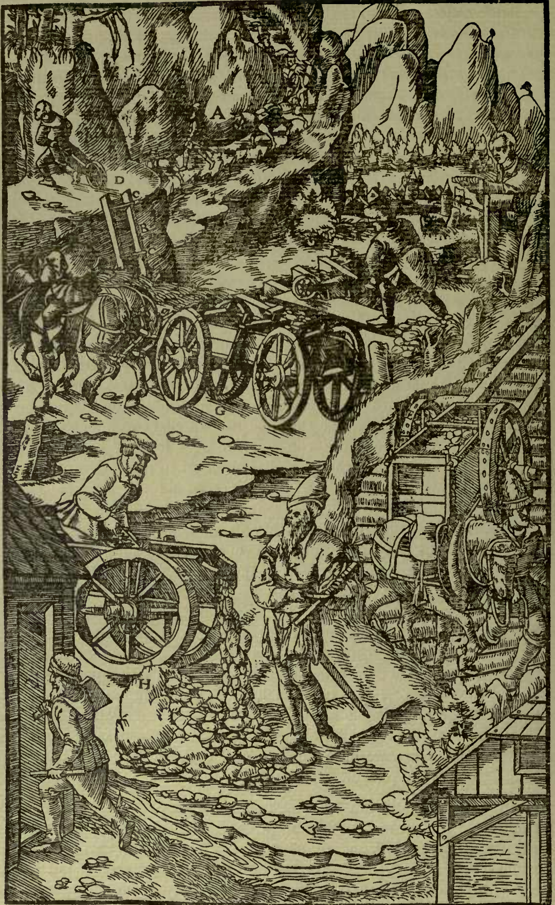
A—HORSES WITH PACK-SADDLES. B—LONG BOX PLACED ON THE SLOPE OF THE CLIFF. C—CLEATS THEREOF. D—WHEELBARROW. E—TWO-WHEELED CART. F—TRUNKS OF TREES. G—WAGON. H—ORE BEING UNLOADED FROM THE WAGON. I—BARS. K—MASTER OF THE WORKS MARKING THE NUMBER OF CARTS ON A STICK. L—BOXES INTO WHICH ARE THROWN THE ORE WHICH HAS TO BE DIVIDED.
