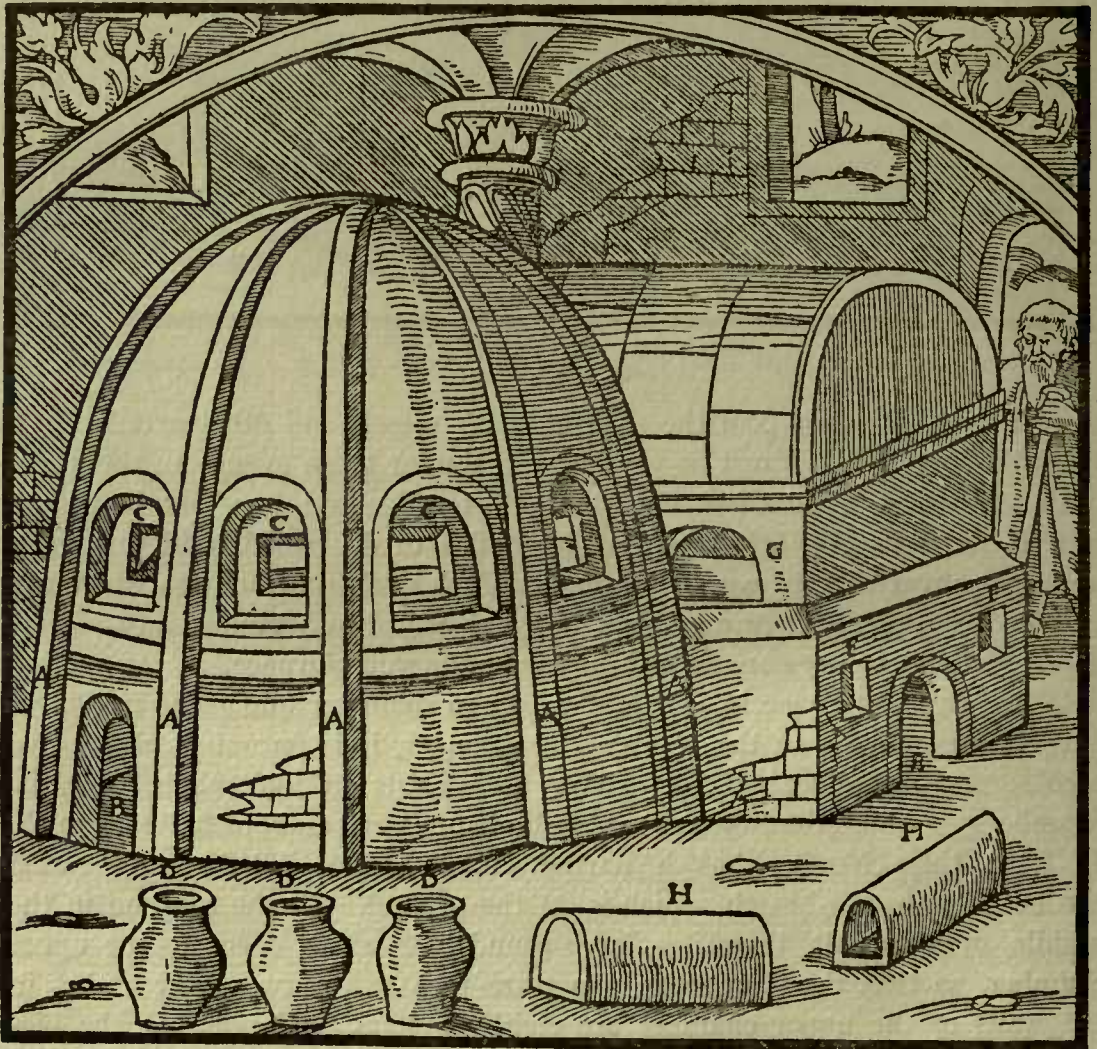
A—ARCHES OF THE SECOND FURNACE. B—MOUTH OF THE LOWER CHAMBER. C—WINDOWS OF THE UPPER CHAMBER. D—BIG-BELLIED POTS. E—MOUTH OF THE THIRD FURNACE. F—RECESSES FOR THE RECEPTACLES. G—OPENINGS IN THE UPPER CHAMBER. H—OBLONG RECEPTACLES.
