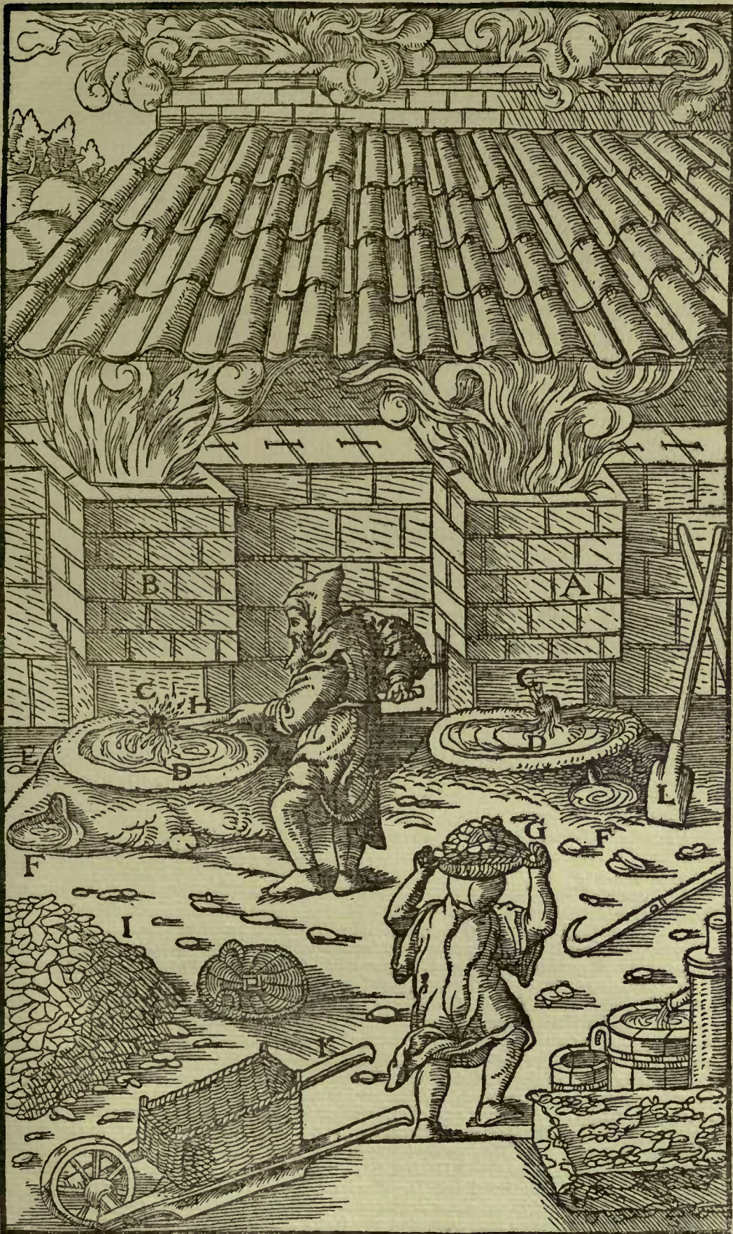
A, B—TWO FURNACES. C—TAP-HOLES OF FURNACES. D—FOREHEARTHS. E—THEIR TAP-HOLES. F—DIPPING-POTS. G—AT THE ONE FURNACE STANDS THE SMELTER CARRYING A WICKER BASKET FULL OF CHARCOAL. AT THE OTHER FURNACE STANDS A SMELTER WHO WITH THE THIRD HOOKED BAR BREAKS AWAY THE MATERIAL WHICH HAS FROZEN THE TAP-HOLE OF THE FURNACE. H—HOOKED BAR. I—HEAP OF CHARCOAL. K—BARROW ON WHICH IS A BOX MADE OF WICKER WORK IN WHICH THE COALS ARE MEASURED. L—IRON SPADE.
