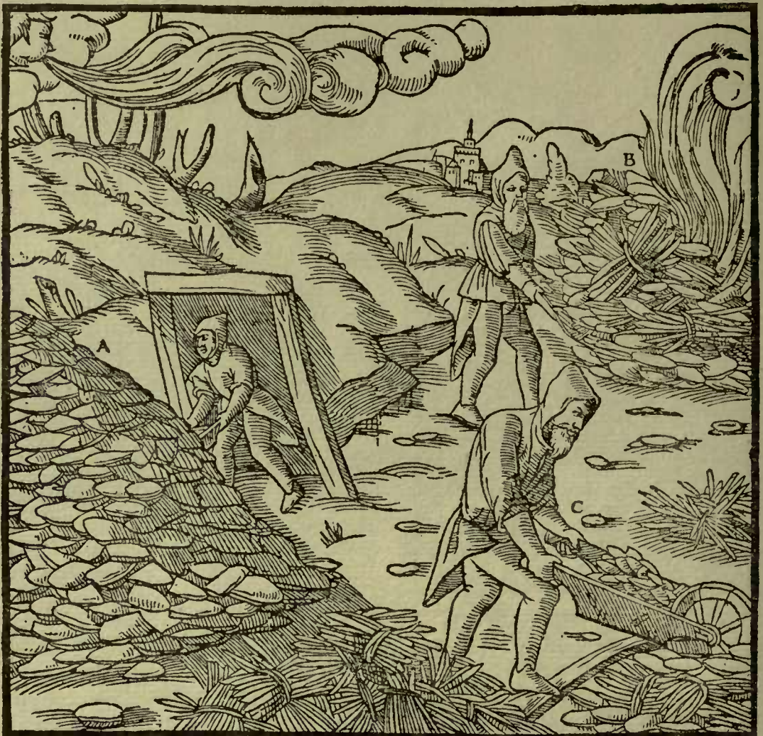
A—HEAP OF CUPRIFEROUS STONES. B—KINDLED HEAP. C—STONES BEING TAKEN TO THE BEDS OF FAGGOTS.
