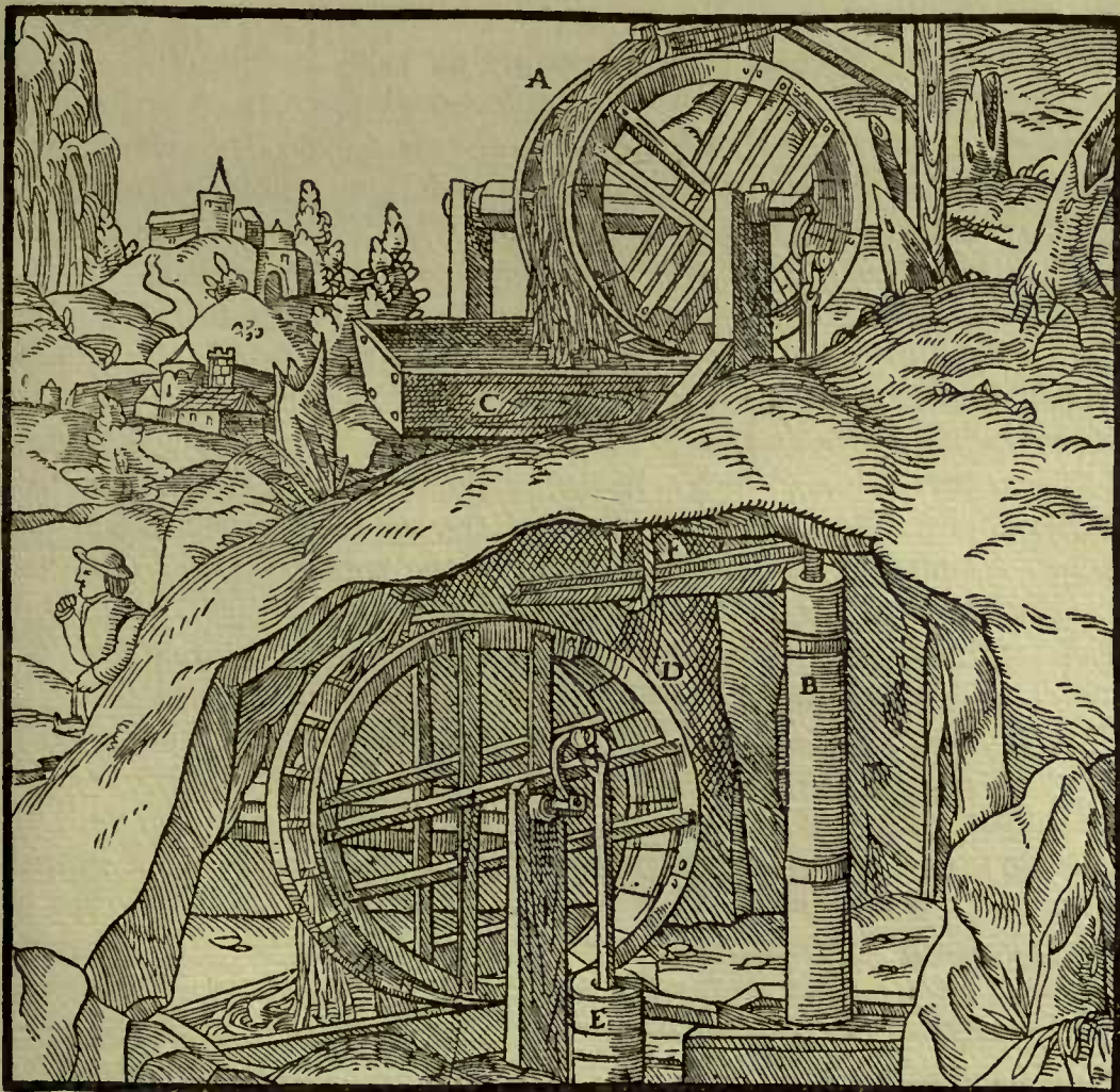
A—WATER WHEEL OF UPPER MACHINE. B—ITS PUMP. C—ITS TROUGH. D—WHEEL OF LOWER MACHINE. E—ITS PUMP. F—RACE.
