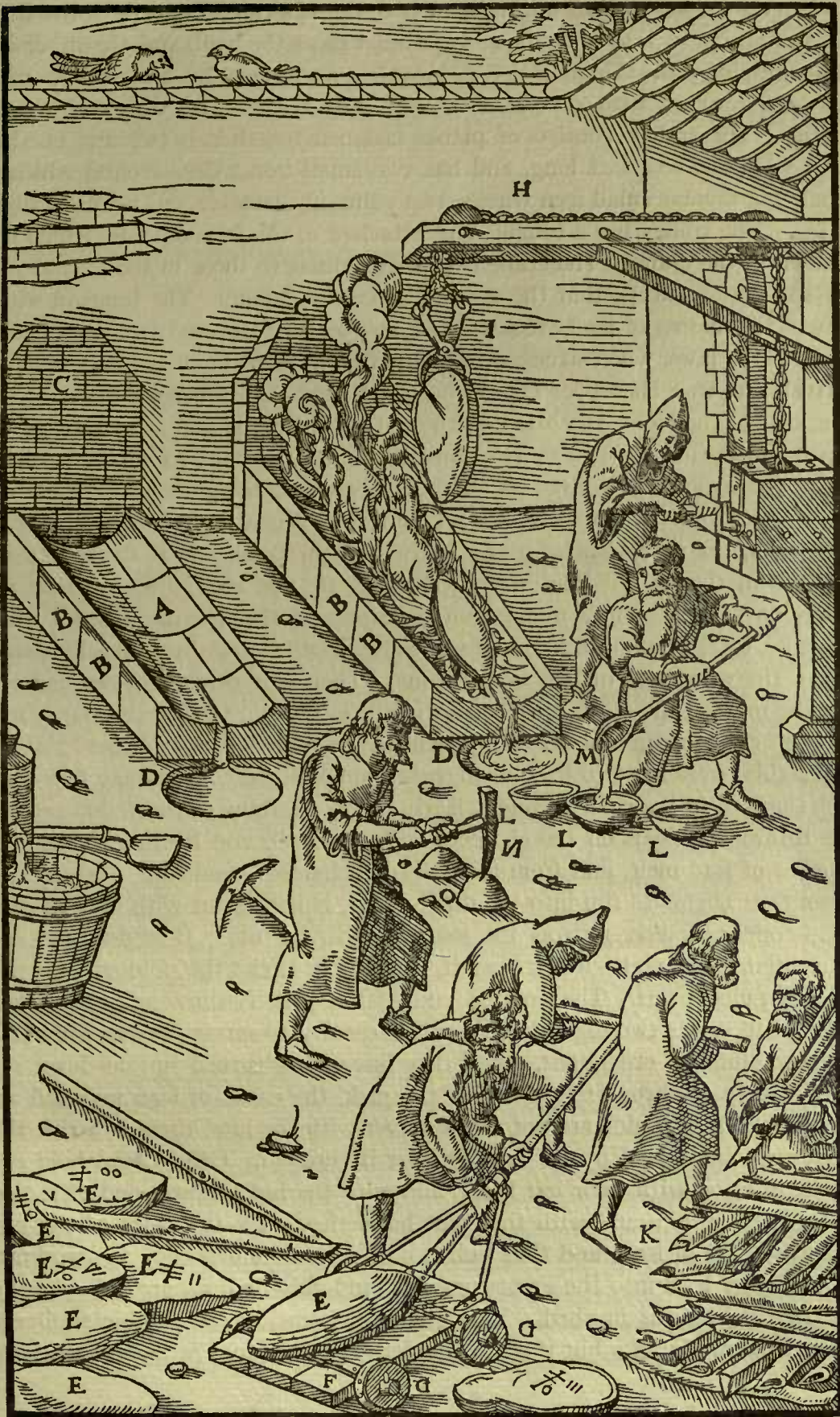
A—HEARTH. B—ROCKS SUNK INTO THE GROUND. C—WALLS WHICH PROTECT THE FOURTH LONG WALL FROM DAMAGE BY FIRE. D—DIPPING-POT. E—MASSES OF LEAD. F—TROLLEY. G—ITS WHEELS. H—CRANE. I—TONGS. K—WOOD. L—MOULDS. M—LADLE. N—PICK. O—CAKES.
