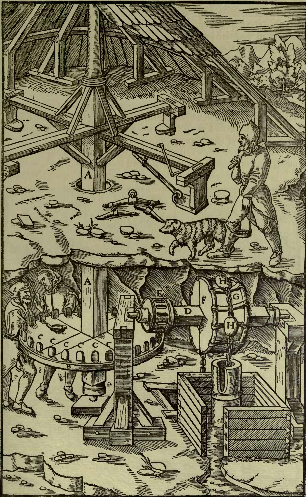
A—UPRIGHT AXLE. B—TOOTHED WHEEL. C—TEETH. D—HORIZONTAL AXLE. E—DRUM WHICH IS MADE OF RUNDLES. F—SECOND DRUM. G—DRAWING-CHAIN. H—THE BALLS.
