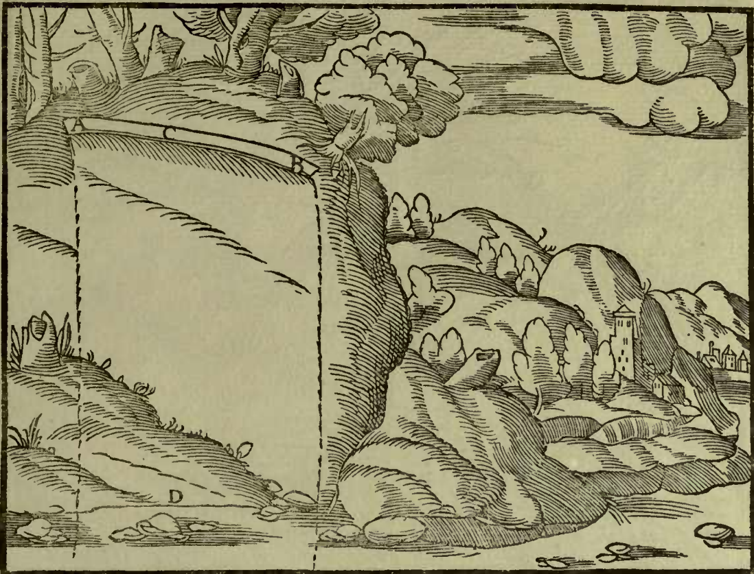
A—THE "BEGINNING" ( origo ). B—THE "END" ( finis ). C—THE "HEAD" ( caput ). D—THE "TAIL" ( cauda ).
