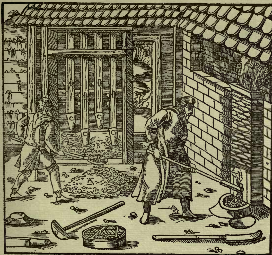
A—CHARCOAL. B—MORTAR-BOX. C—STAMPS.
