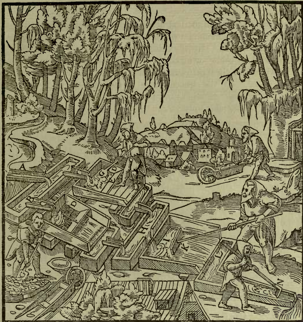
A—LAUNDER. B—CROSS TROUGH. C—TWO SPOUTS. D—BOXES. E—PLATE. F—GRATING. G—SHOVELS. H—SECOND CROSS TROUGH. I—STRAKE. K—WOODEN SCRUBBER. L—THIRD CROSS TROUGH. M—LAUNDER. N—THREE-TOOTHED RAKE.
