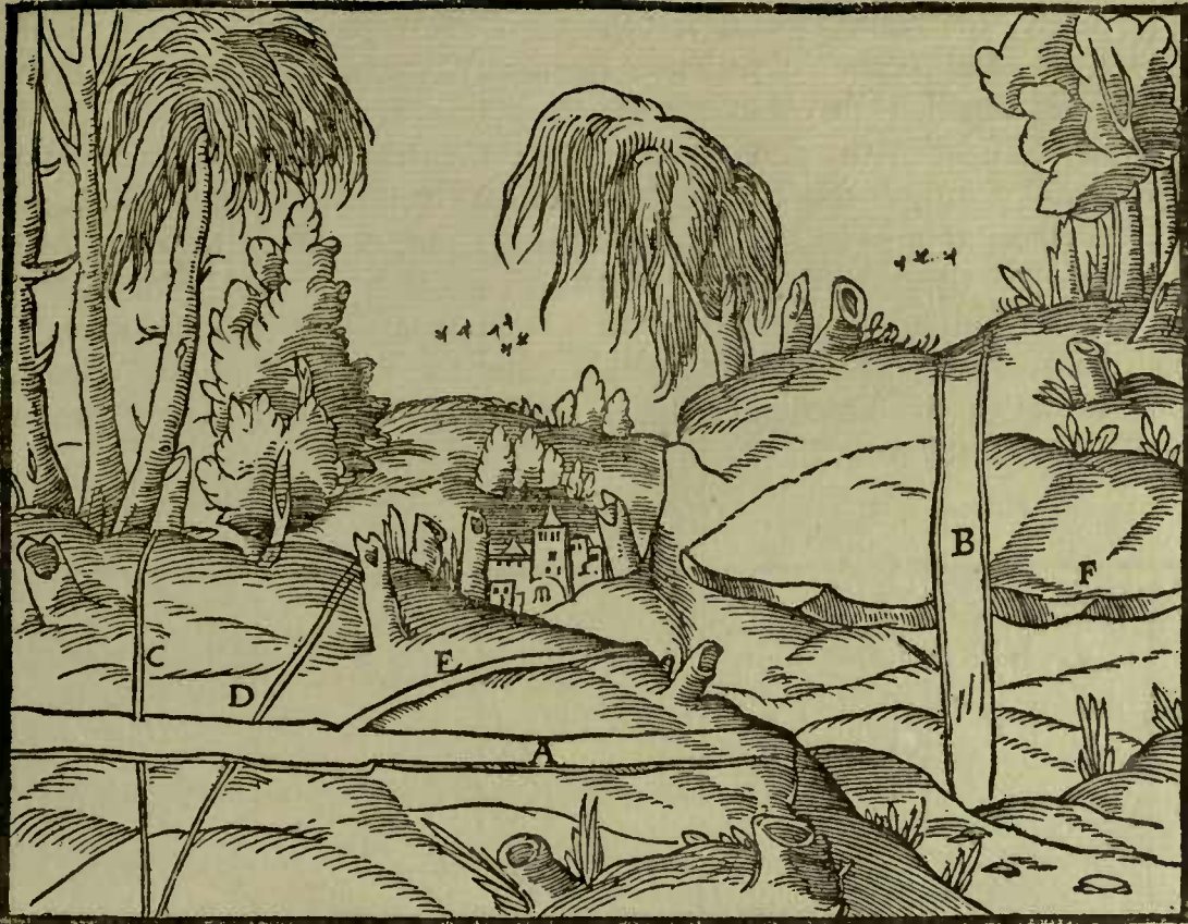
A, B—VEINS. C—TRANSVERSE STRINGER. D—OBLIQUE STRINGER. E—ASSOCIATED STRINGER. F— Fibra dilatata .
