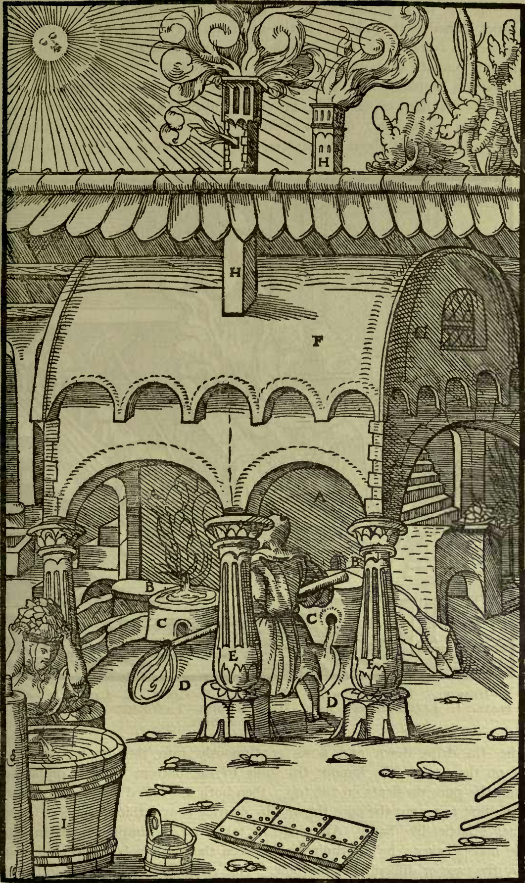
A—FURNACES. B—FOREHEARTHS. C—THEIR TAP-HOLES. D—DIPPING-POTS. E—PILLARS. F—DUST-CHAMBER. G—WINDOW. H—CHIMNEYS. I—TUB IN WHICH THE COALS ARE WASHED.
