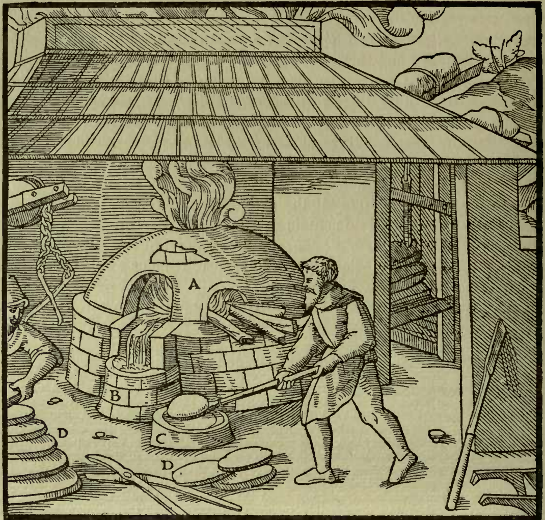
A—FURNACE. B—FOREHEARTH. C—DIPPING-POT. D—CAKES.
