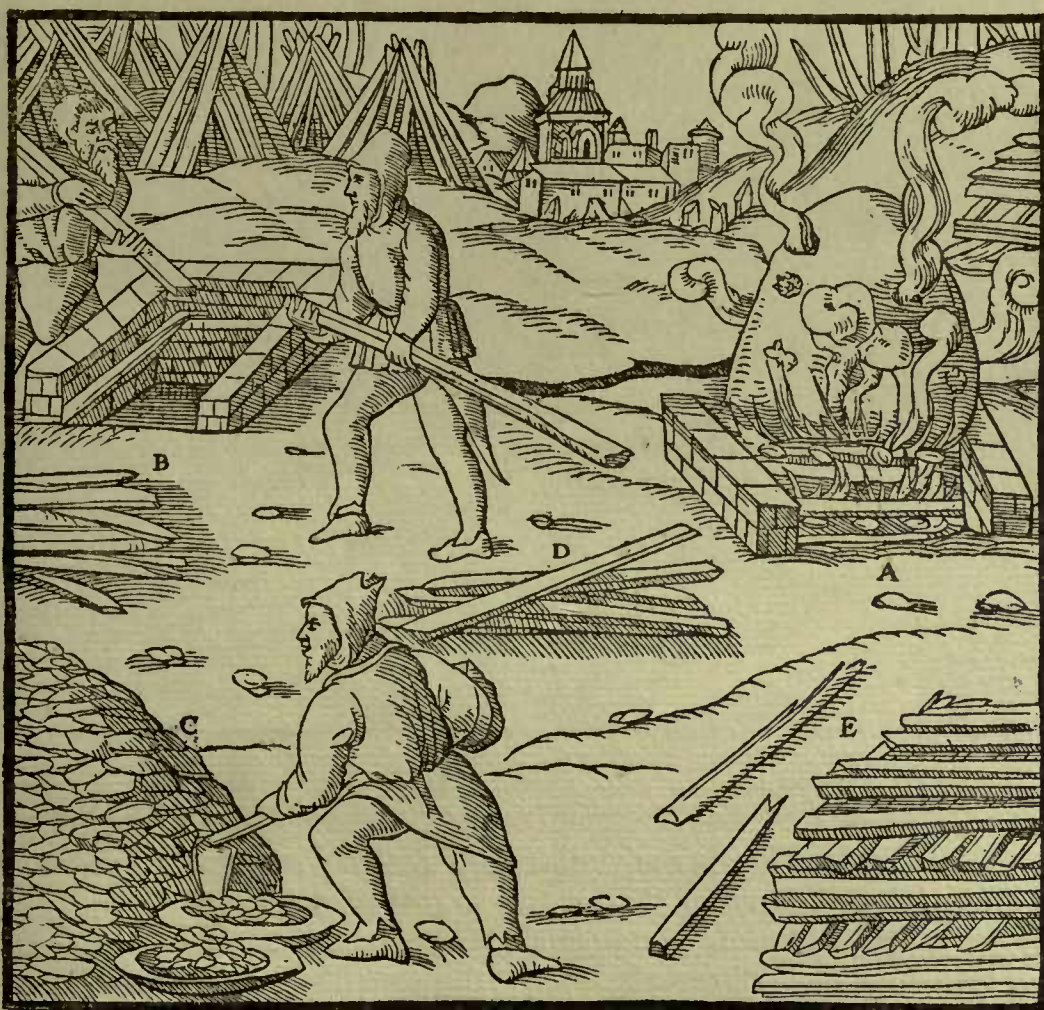
A—LIGHTED PYRE. B—PYRE WHICH IS BEING CONSTRUCTED. C—ORE. D—WOOD. E—PILE OF THE SAME WOOD.
