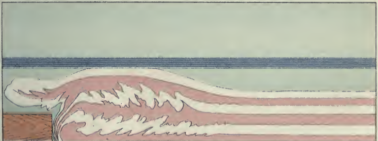
Fig. 4. Pie Paste. Compression restricted to the lower Strata under a rigid upper one.
