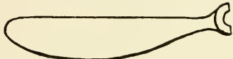
Sketch of the Chauvière blade. The round part is the leading edge.
