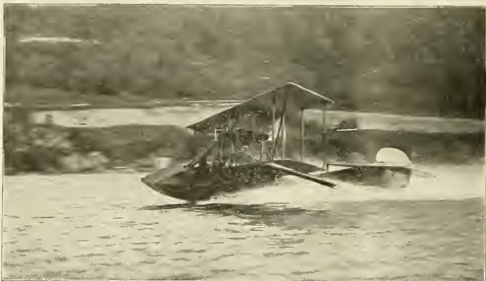
G. M. Heckscher operating his new Curtiss racing flying boat on Lake Keuka at sixty miles an hour. Note the elevator held down to keep the machine in the water and also the absence of spray in front of the boat, which is just planing on the top of the water.
