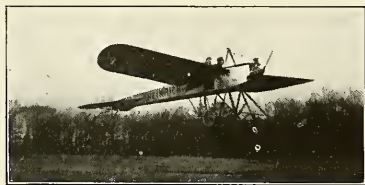
Starting on a flight with a passenger on a 30 H. P. Heinrich Monoplane
