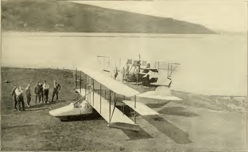
A scene at the Curtiss flying school at Hammondsport, New York, showing two of the latest Curtiss flying boats drawn up on the beach. The machine in the foreground is the latest Curtiss Flying Boat, purchased by Marshall E. Reid, the well-known aviator, who is seen seated in it. The machine in the background is one of the school flying boats with hinged hood, which is used as a gangplank and permits boarding or disembarking at a pier so that there is no longer any need of drawing the machine up on to the land when taking passengers on or off.
