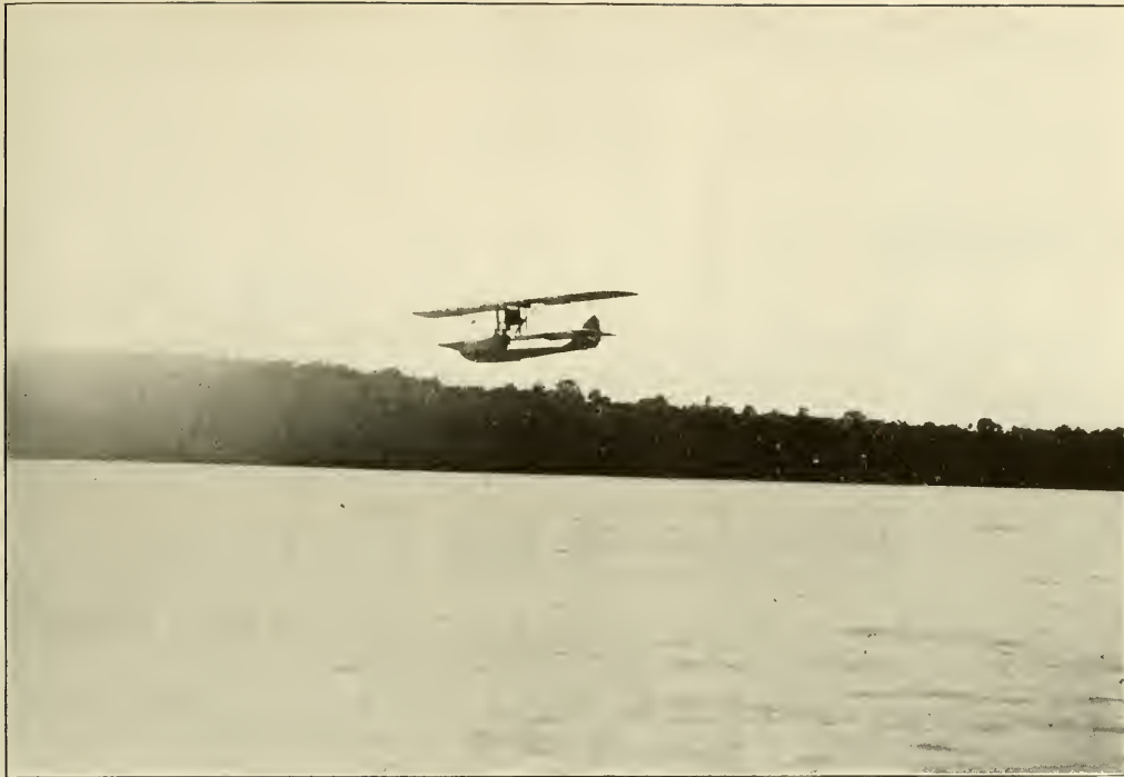
W. E. Johnson and W. T. Thomas airing a Thomas Flying Boat over Conesus Lake, N. Y. This boat is of two-ply planking with sheet steel bottom and has a collapsible spray shield. Its speed with passenger is 60 miles an hour. During the summer months, Mr. Johnson carried a great number of passengers over the Lake which netted quite a large sum of money in fares.
