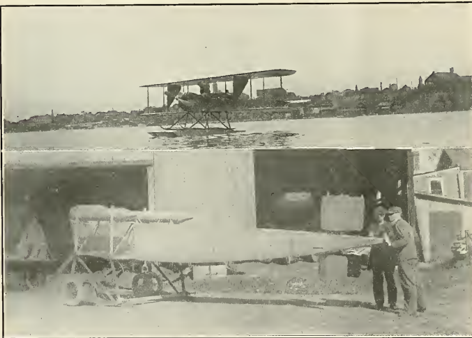
Model "H" Burgess tractor biplane, a number of which have been ordered by the United States Signal Corps, and which have recently passed most successful tests. The hydroplanes on which the tractors are mounted are of special type. The machine is easily convertible into a land machine, the work being accomplished in less than 15 minutes. The whole machine can be taken down ready for shipment inside of half an hour. The speed of the machine is increased over the 1912 type by three or four miles on account of the refinements in construction and the use of the Burgess linen. It now has a speed ranging from 45 to 60 miles per hour.
