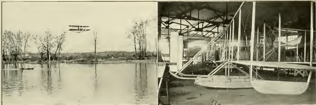
The picture on the left shows Mr. Orville Wright flying a new Wright hydro-aeroplane above the Miami River, Dayton; while the picture on the right shows a close view of the new model C-H single pontoon Wright.
