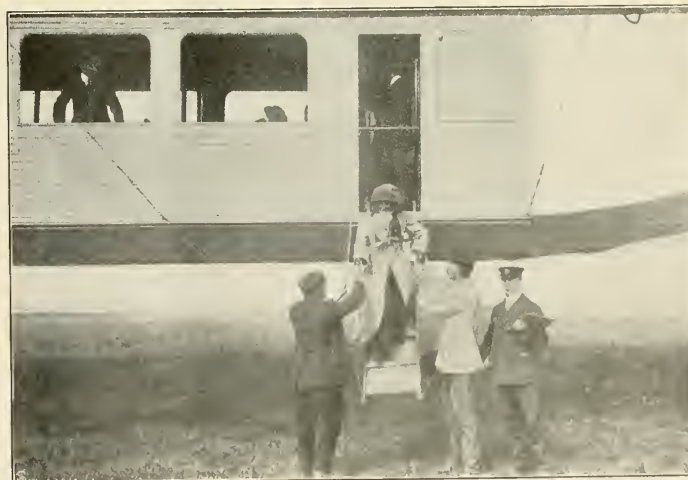
Descending the gangplank. The collapsible gangway of a Zeppelin is raised by wires until it becomes the closed door to the cabin.
