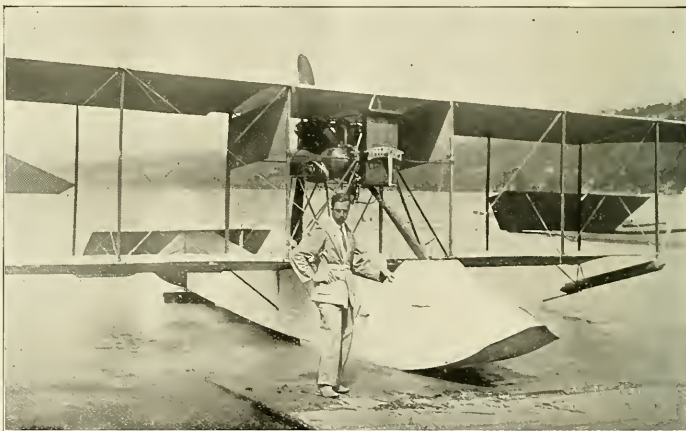
L. A. Vilas, of Chicago, and his new Curtiss flying boat, which is one of the finest finished craft ever constructed, having the metal work, braces, engine section, controls and other parts silver plated. The neat bucket seats are upholstered in soft dove-colored corduroy; in fact, the whole of the cockpit is fitted out like a luxurious landaulet, while the boat and all the woodwork have been painted with the same care and finish as is found on high-class automobiles.
