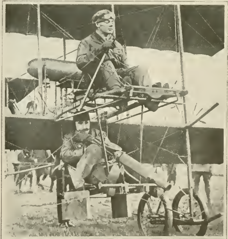
TO SHOW THE POSITIONS OF THE GUNNER AND THE PILOT THE GUN MOUNTED ON A 4-HP GRAHAME-WHITE BIPLANE.
