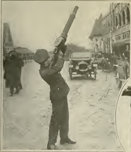
THE WEAPON USED ON THE GROUND TRYING TO HIT AN AEROPLANE WITH THE LEWIS AIR-COOLED MACHINE-GUN.
