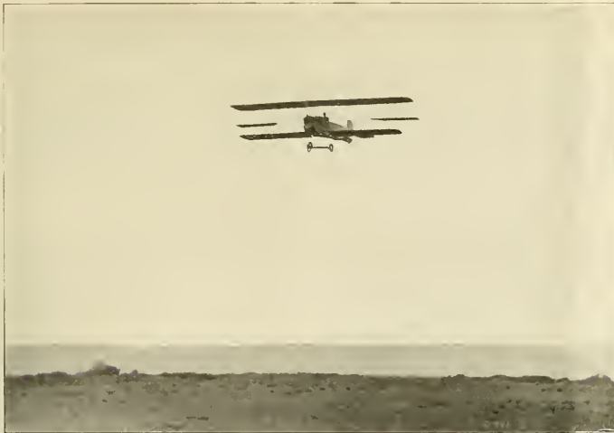
Glenn H. Curtiss flying the new Curtiss military tractor biplane at San Diego, Cal. The planes of the machine are slightly swept back in a manner similar to the Lohner Arrow biplane.
