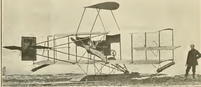
The above photograph shows the new device for stabilizing aeroplanes invented by H. C. Fiske, of Stamford, Conn. It consists of a disk of canvas 7 ft. in diameter with the sides curved upward 10 lbs. from the horizontal at the extremities. The device weighs 11 lbs. and the form and method of mounting it is plainly shown in the photographs. William S. Luckey recently tried it out in a number of trial flights in which he declared it to be very satisfactory. He states that he found under medium speed the aeroplane was very steady without using the ailerons and that it was also effective at high speeds in straight flights and medium large circles. He also stated that the machine banked and handled very nicely in calm air and in a wind of 30 miles velocity. The curve of the stabilizer is such that if the machine starts to drop aside the air banking up against the lower side of the disk will bring it back to level. When making a turn the machine banks automatically, for the lateral drift due to centrifugal action brings air pressure against the side of the disk and causes the plane to lift on the outer end. The lower picture shows a Curtiss hydroaeroplane fitted with a disk stabilizer, while the upper picture shows it in flight without using the ailerons.
