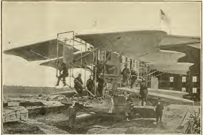
The picture above shows the flying machine recently constructed by Captain Matthew A. Batson, U.S.A. (Retired) for the purpose of endeavoring to fly across the Atlantic Ocean. It was built at Dutch Island, near Savannah, Ga., and weighs about 5,000 lbs., and the inventor of it claims an additional lifting capacity of two tons. The machine is equipped with twelve large wing planes, one pair having a spread of 32 1/2 ft. and four pair with a spread of 37 1/2 ft., while a sixth pair has a spread of 30 ft. The wings are designed with the purpose of guiding the air currents inwardly toward the body of the machine and there banking them under the base portion of the wings, which are concaved underneath and carried back along the chassis so that the currents of air are conducted along the parts nearest the chassis. Any wing or set of wings or all twelve may have their angle of incidence changed at the will of the pilot by the turn of a wheel while the machine is in full flight. The machine is equipped with three six-cylinder engines installed in the floor of the pilot house. These engines are supposed to supply 350 H. P. to drive the propellers at 1,000 revolutions per minute. Any one of the engines may be thrown out of or into action by the operation of a clutch. The cabin of the machine is 27 ft. long and is constructed of cypress paneling 3/4 of an inch thick, over which is a covering of canvas. The life boat is made of three-ply cypress and ash with inter-layers of canvas. The length of the machine is 74 ft. and of the boat 33 ft. AIRCRAFT has heard of no flights being made by this machine as yet.
