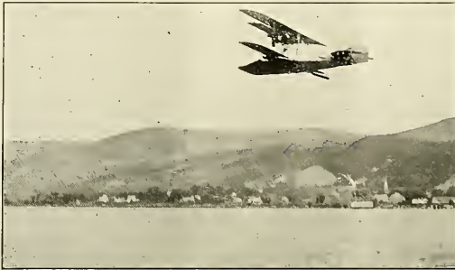
The sturdy Curtiss Flying Boat in flight. Note the substantial hull and generous size of main planes, elevators and rudder. Attention is also called to the position of the motor high up between the planes.
