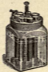
FIG. 31.—SINGLE-FLUID ZINC-CARBON CELL.
