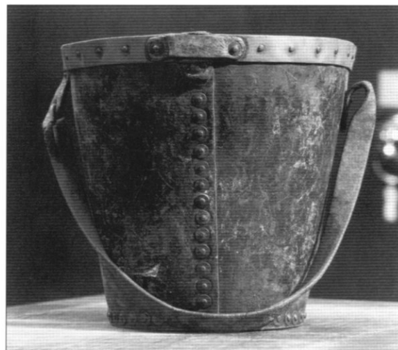
ABOVE A leather bucket typical of the Napoleonic period with copper rivet fittings and a copper ring. These were used for dipping the sponge prior to swabbing the bore of the gun. The excess water was normally wiped off because, if the sponge were too damp, this could affect the firing of the gun. It is a common misconception that the sponge was used to clean the bore of the gun. While this was one function, the main function was to put out burning embers in the gun barrel before loading a new charge and thus preventing a premature explosion. (Museum of Naval Firepower)
