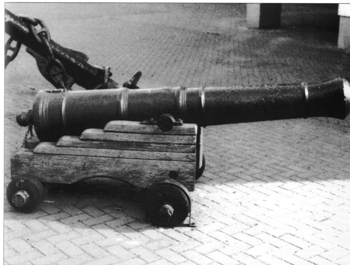
BELOW An early pattern Armstrong Frederick gun, in this case a 12-pdr. The trunnion on this weapon is marked with the letter B indicating that it was cast by William Bengel. The carriages are reproductions. (Museum of Naval Firepower)
