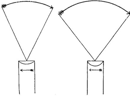
*Fig. 13.*—*a*, Objective with small angle; therefore small field of view, good magnification and illumination. *b*, Wider-angled objective; large external field, loss of magnification and illumination.
