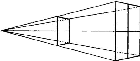
*Fig. 17.*—Illustrating loss of light by distance of lamp from object.
