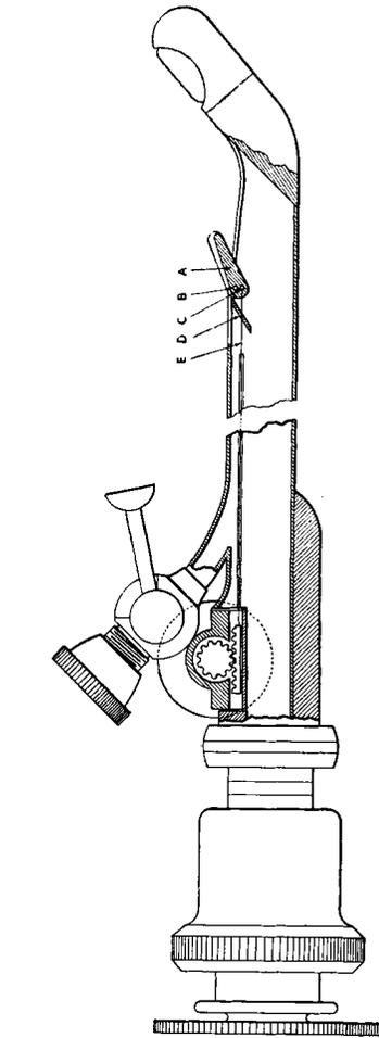
*Fig. 117.*—Single catheterizing cystoscope. A, Albarran lever; B, Pin on which the lever works; C, Pinhole through which the wires pass—pushing in order to lift the lever, and pulling to lower it; D, Sloping guide to direct ureteric catheter towards the lever; E, Wire connecting lever with rack.
