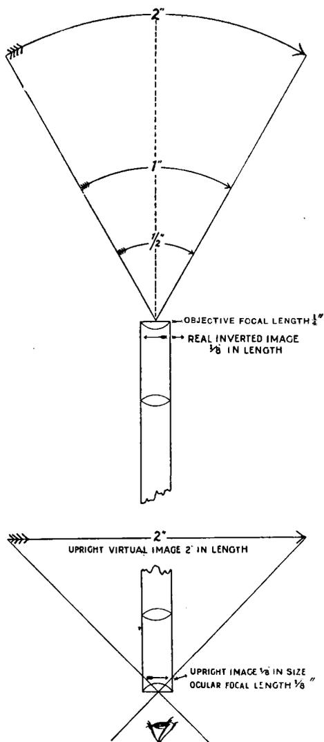
*Fig. 15.*—Diagram illustrating the properties of the telescope.
