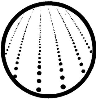
*Fig. 22.*—Lines of parallel dots on a printed card seen through the cystoscope, showing the effects of foreshortening and distortion.
