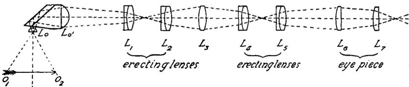
*Fig. 21.*—Lens system used in instrument made by the Genito-Urinary Manufacturing Co., London.  $O_1, O_2$ , The object;  $L_0, L_0'$ , Two parts of objective separated by a roof prism;  $L_1, L_2, L_3, L_4, L_5$ , Transporting system;  $L_6, L_7$ , Eye-piece.
