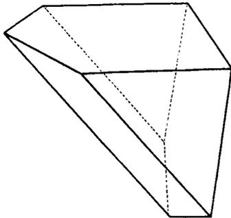
*Fig. 26.*—Amici's 'roof' prism.
