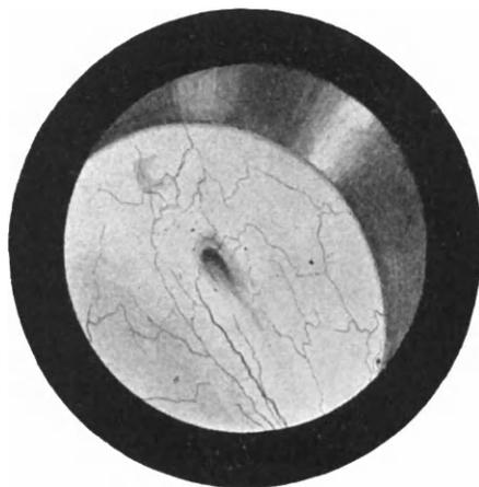
*Fig. 31.*—Ellipse of field of view cut off owing to bend in the telescope.
