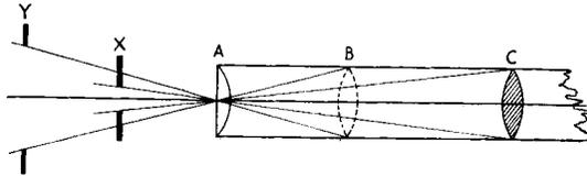
*Fig. 20.*—Diagram illustrating the respective size of the entrance pupil in the new and the old lens systems.
