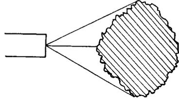
*Fig. 16.*—Diagram to indicate that the portions of a convex object closest to the prism are more highly magnified than those which are more remote.
