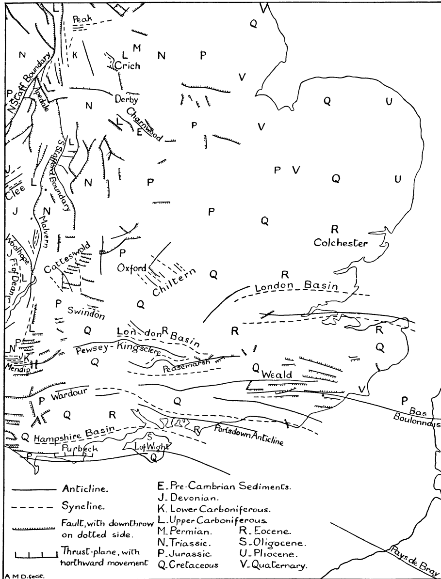
Fig. 8. Tectonic Map of the British Isles.—Section VIII.—England (Central, Southern and Eastern). Malvernian, Charnian and Armorican systems. The London Basin is seen to be composed of two separate synclines, not in line; the connexion between them is obscure owing to slightness of dip. A. M. D.
