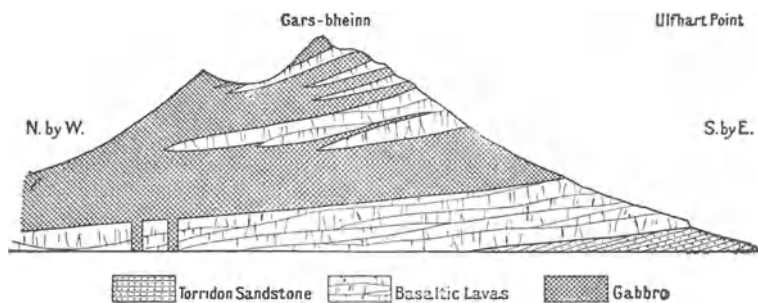
Fig. 63. Section through Gars-bheinn, Skye, to illustrate alternations of basaltic lavas and gabbro, due to the successive intrusions of the latter rock having followed different bedding-planes in the lavas. Scale: 2 inches to 1 mile or 1:126,720.
