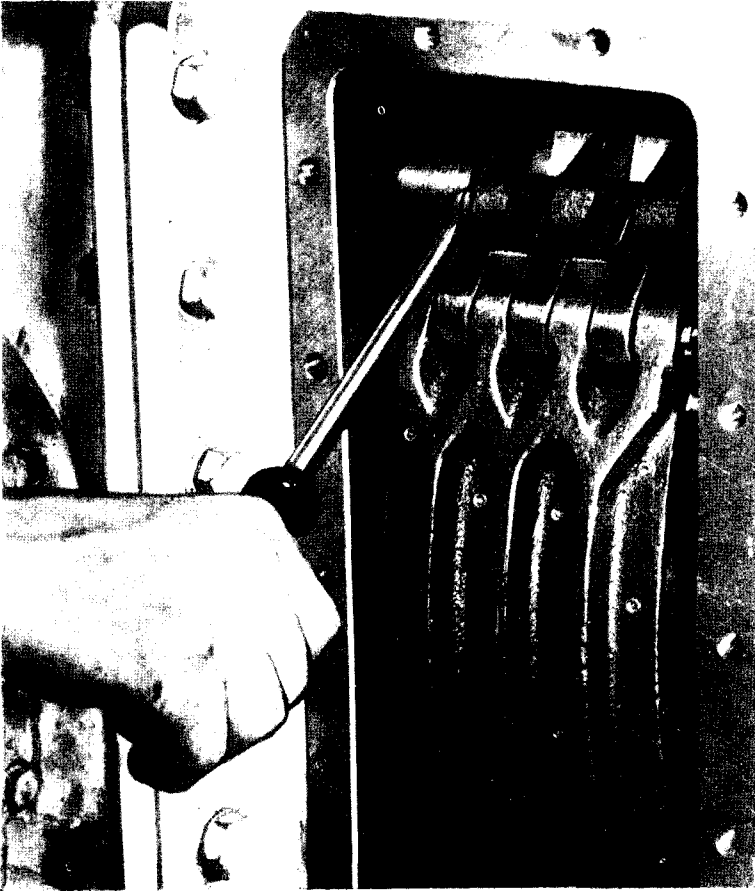
Figure 78—Removing Link Pin from Cam
