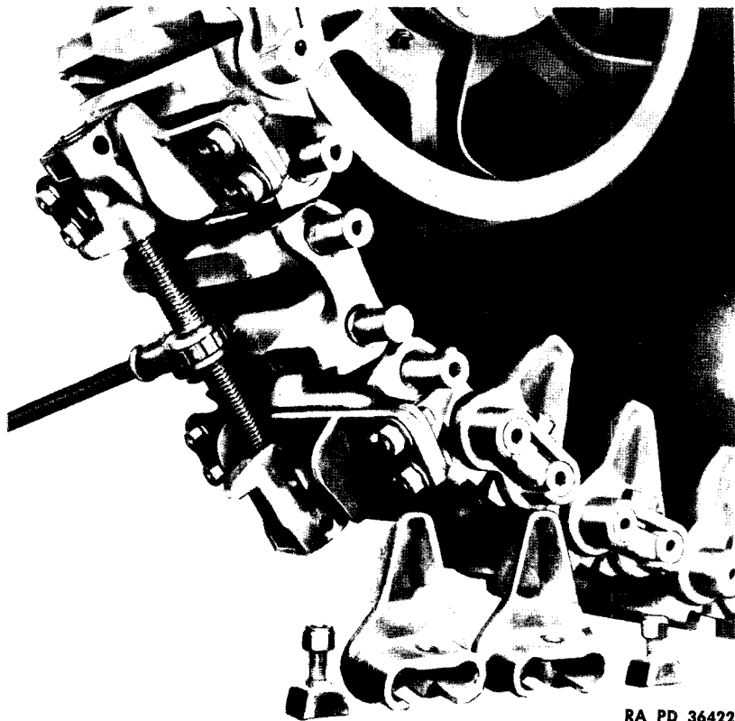
Figure 88—Replacing Dead Track Block
