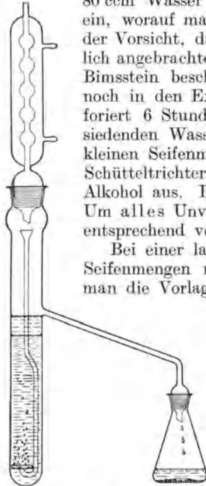
Abb. 6. Perforationsapparat.
