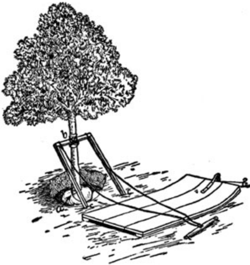
RIG FOR MOVING TREE
