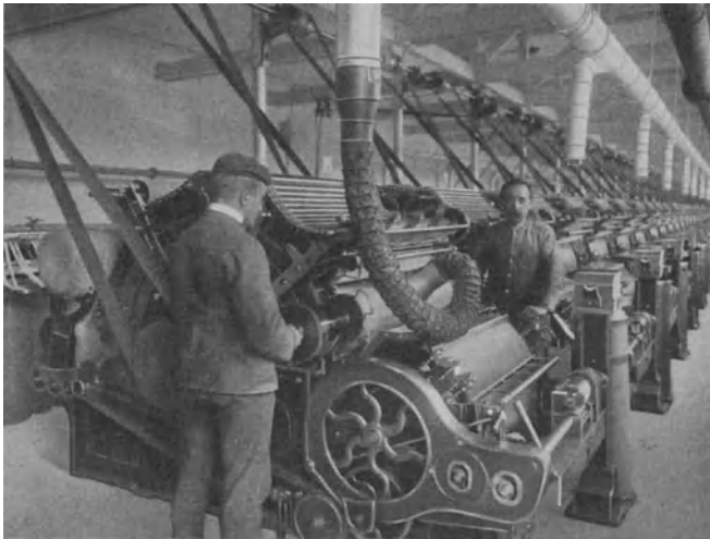
Abb. 82. Karden-Entstaubungsanlage (B. Schilde, A.-G., Hersfeld).
