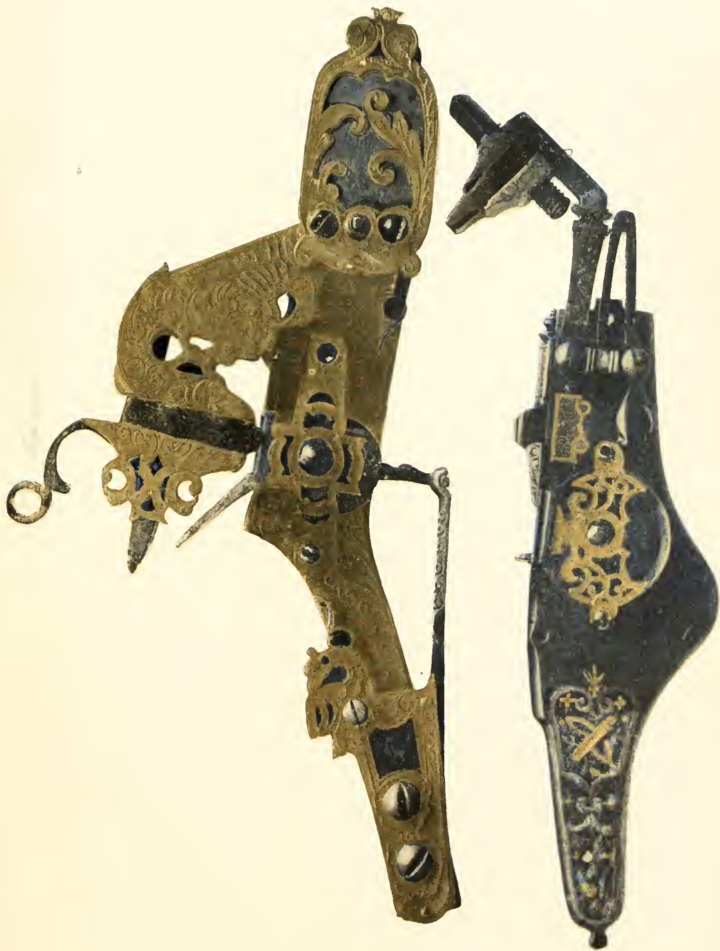
PLATE VIII.—Wheel-lock of bright steel, with engraved and pierced brass. German, 17th Century.
