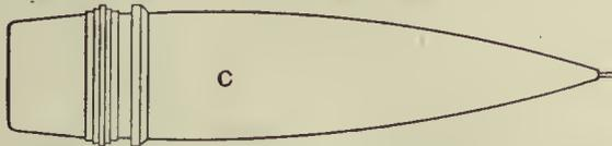
German 17 cm H.E. Shell, 4 7 calibres long, streamlined with False Cap, Nose Fuze, 2 Driving bands & decoupling ring, about 11 c.r.h.
