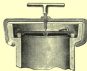
Fig. 345.—Doulton's Clip for Holding Stopper in End of Drain.
