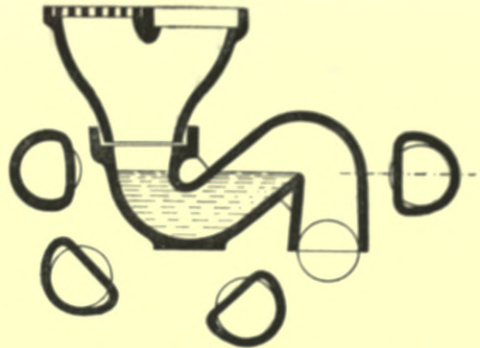
Fig. 380.—Green's Soil-pipe Interceptor.
