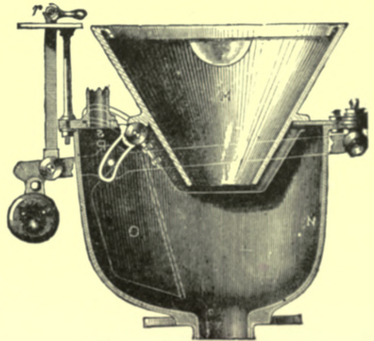
Fig. 285. —Section of Pan-closet.
