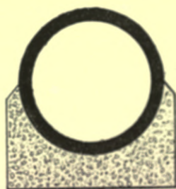
Fig. 404. — Concrete Cradle for Pipes.
