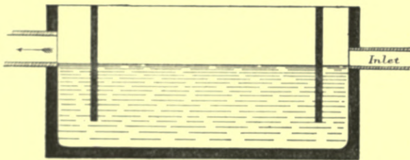
Fig. 385. — Grease-trap for Moderate-sized House.
