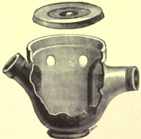
Fig. 389.—Bolding's "Simplex" Grease-trap.
