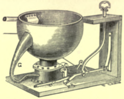
Fig. 284. —View of Bramah's Water-closet.
