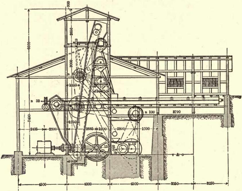
FIG. 66.—TRANSVERSE SECTION OF SEPARATION WORKS, NEUNKIRCHEN, GERMANY.
