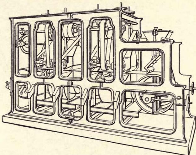
FIG. 35.—HUMBOLDT-WETHERILL CROSS-BELT SEPARATOR.
