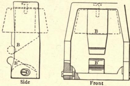
FIG. 31.—DETAIL OF PRIMARY MAGNET, KNOWLES SEPARATOR.
