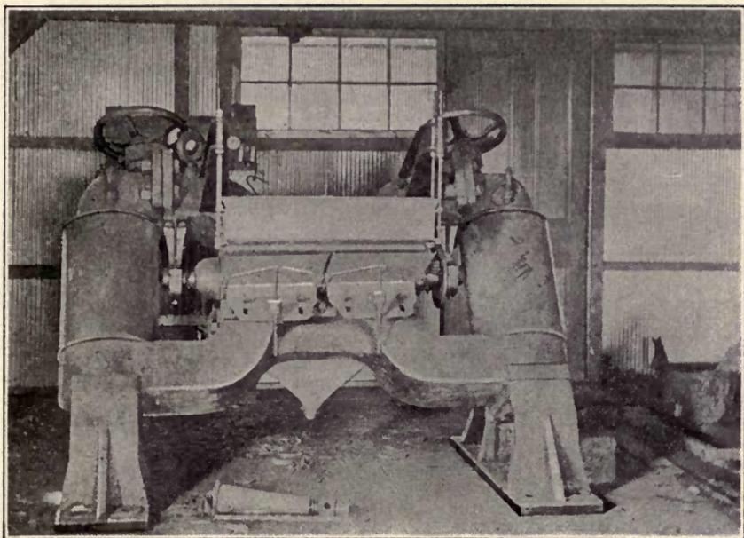
FIG. 77.—MOTORTYPE SEPARATOR, PLANT NO. 2, SULPHIDE CORPORATION.
