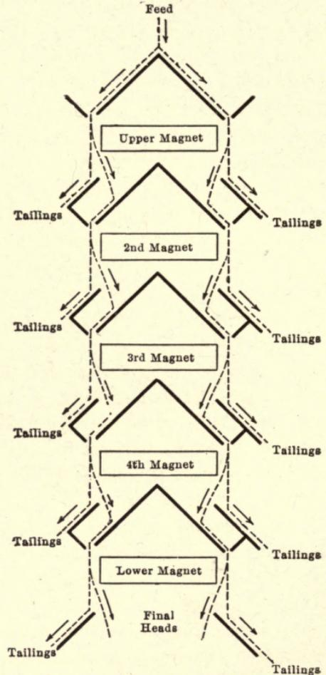
FIG. 14.—CLEANING MAGNETS,
