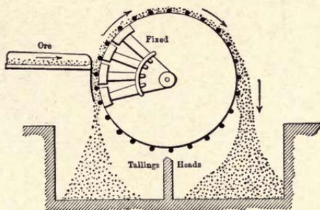
FIG. 28.—THE HEBERLE DRY SEPARATOR.
