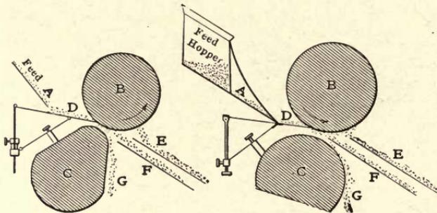
FIG. 36.—CROSS-SECTIONS OF MAGNETS, MECHERNICH SEPARATOR.
