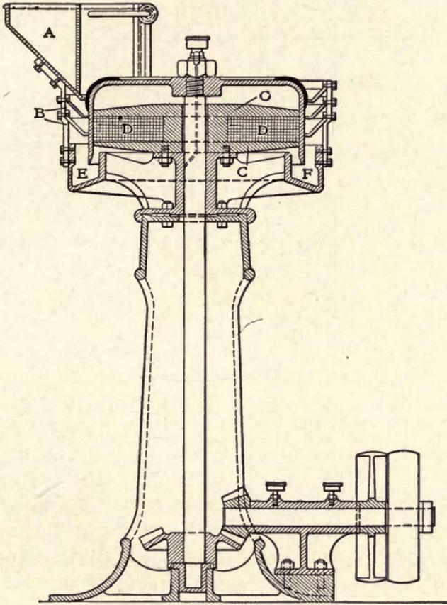
FIG. 4.—THE GRONDAL TYPE II SEPARATOR.
