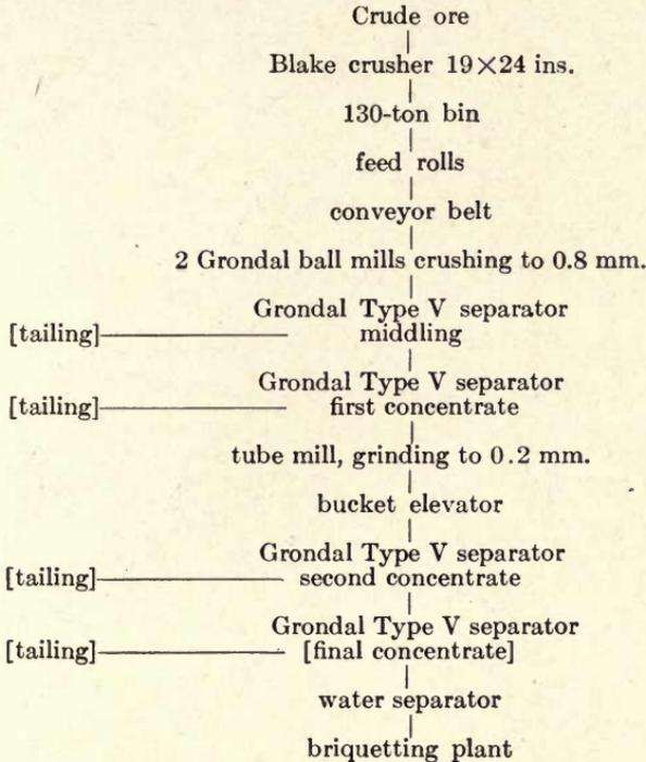
cent. iron. The tailing product carries from 12.7 to 14.6 per cent. iron.<sup>1</sup> The plant is operated by 6 men, and requires 20 H.P. and 200 liters of water per minute. The mill produces 20 metric tons of concentrate per day.
