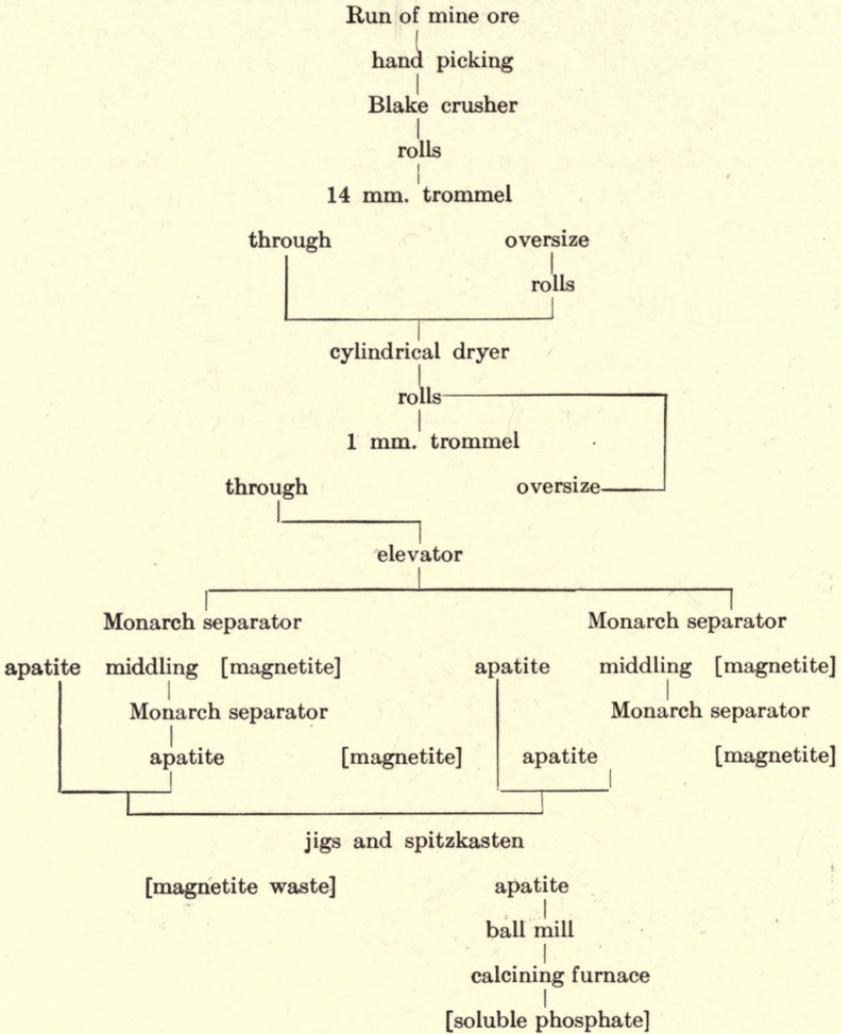
in 1903 is in operation on small ores; the Wenstrom separator is employed. The run of mine ore is subjected to hand picking, a clean magnetite product carrying up to 60 per cent. being thrown out and sent directly to the furnaces. The ore is lifted by elevator to the top floor of the mill and dumped into a bin of 1.5 cu. yds. capacity. The mill flow sheet follows on page 106.<sup>1</sup>
