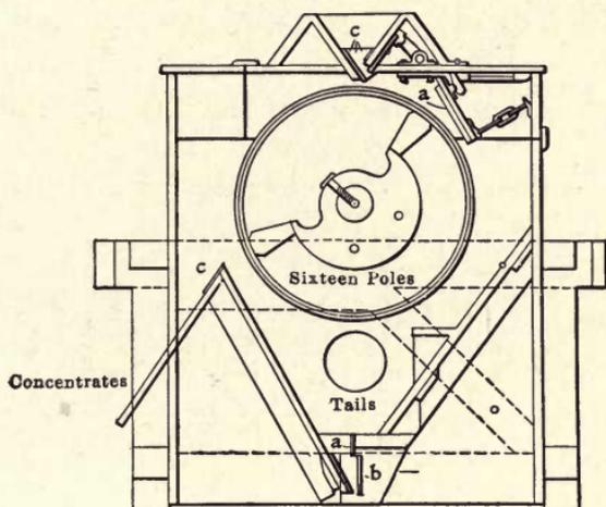
FIG. 16.—THE BALL-NORTON SINGLE-DRUM SEPARATOR.
