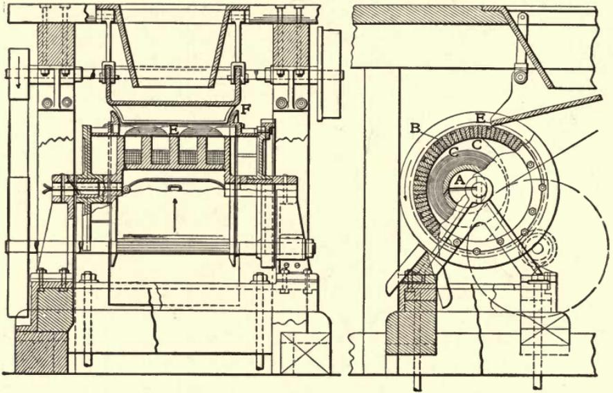
FIG. 17.—THE WENSTROM SEPARATOR.
