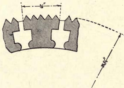
FIG. 41. — DETAIL OF SEPARATING SHELL, UPPER DRUM, PAYNE SEPARATOR.
