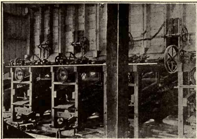
FIG. 60.—DINGS SEPARATORS AT KOKOMO, COLORADO.
