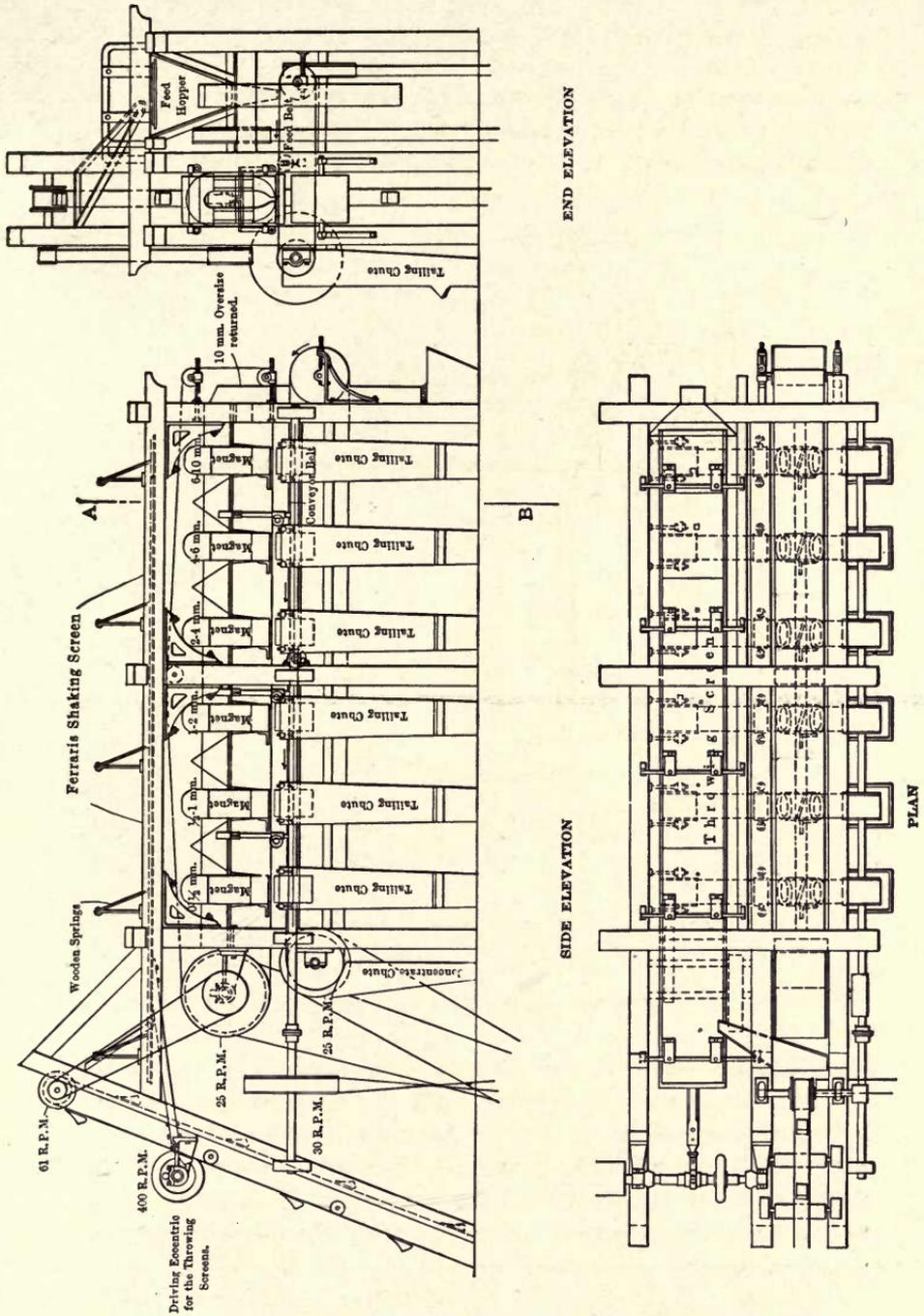
FIG. 26. — THE FERRARIS CROSS BELT SEPARATOR.
