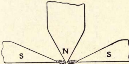
FIG. 45. — SHOWING CONCENTRATION OF MAGNETIC FIELD.
