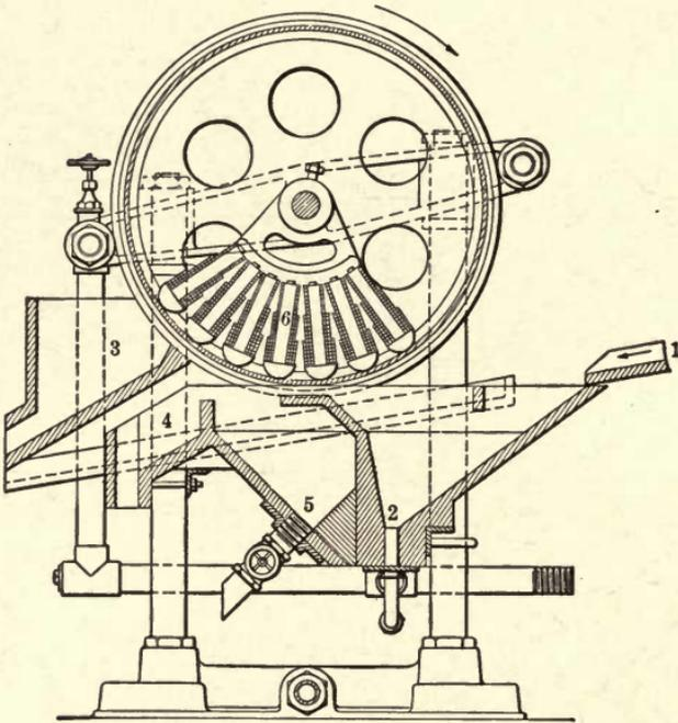
FIG. 6.—THE GRONDAL TYPE V SEPARATOR.
