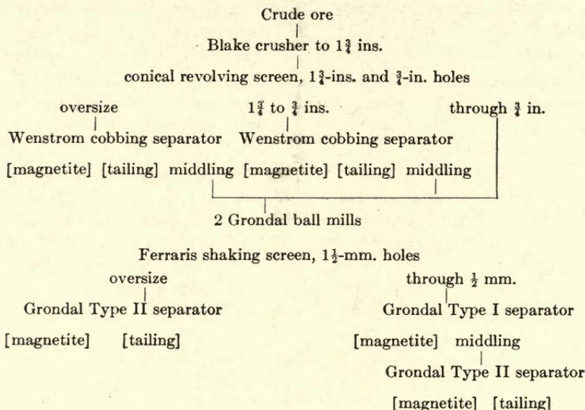
cent. iron. Each separator puts through ¼ metric ton per hour; the magnets are excited by 3 amperes at 90 volts. Fourteen men and 60 H.P. are required to operate the plant. The water used amounts to 600 liters per minute.<sup>1</sup>
