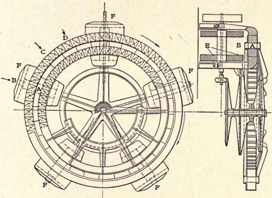
FIG. 12.—THE FORSGREN SEPARATOR.
