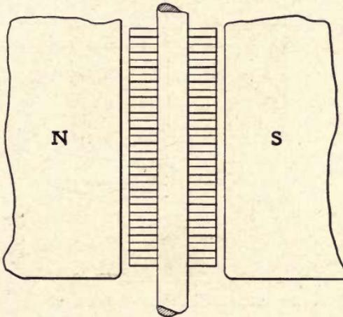
FIG. 9.—DETAILS OF MAGNET ROLLER, WETHERILL TYPE F SEPARATOR.
