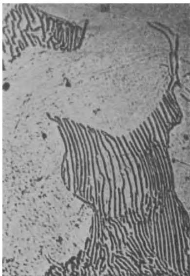
Abb. 4. Ferrit (hell) + Perlit (lamellares Aggregat).
